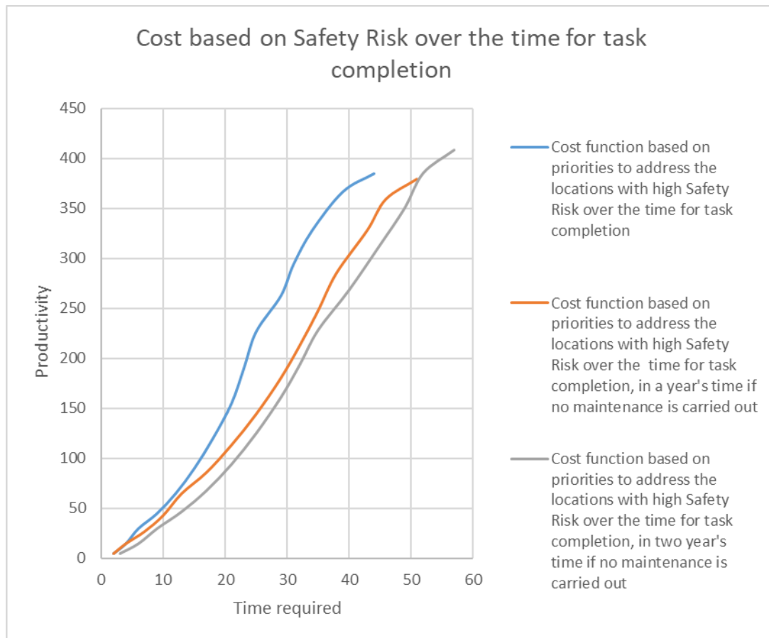
Figure 12: Changes in resource utilisations if no maintenance is carried out, based on Consequences of not doing the tasks – Safety Risk over the time required to complete task
