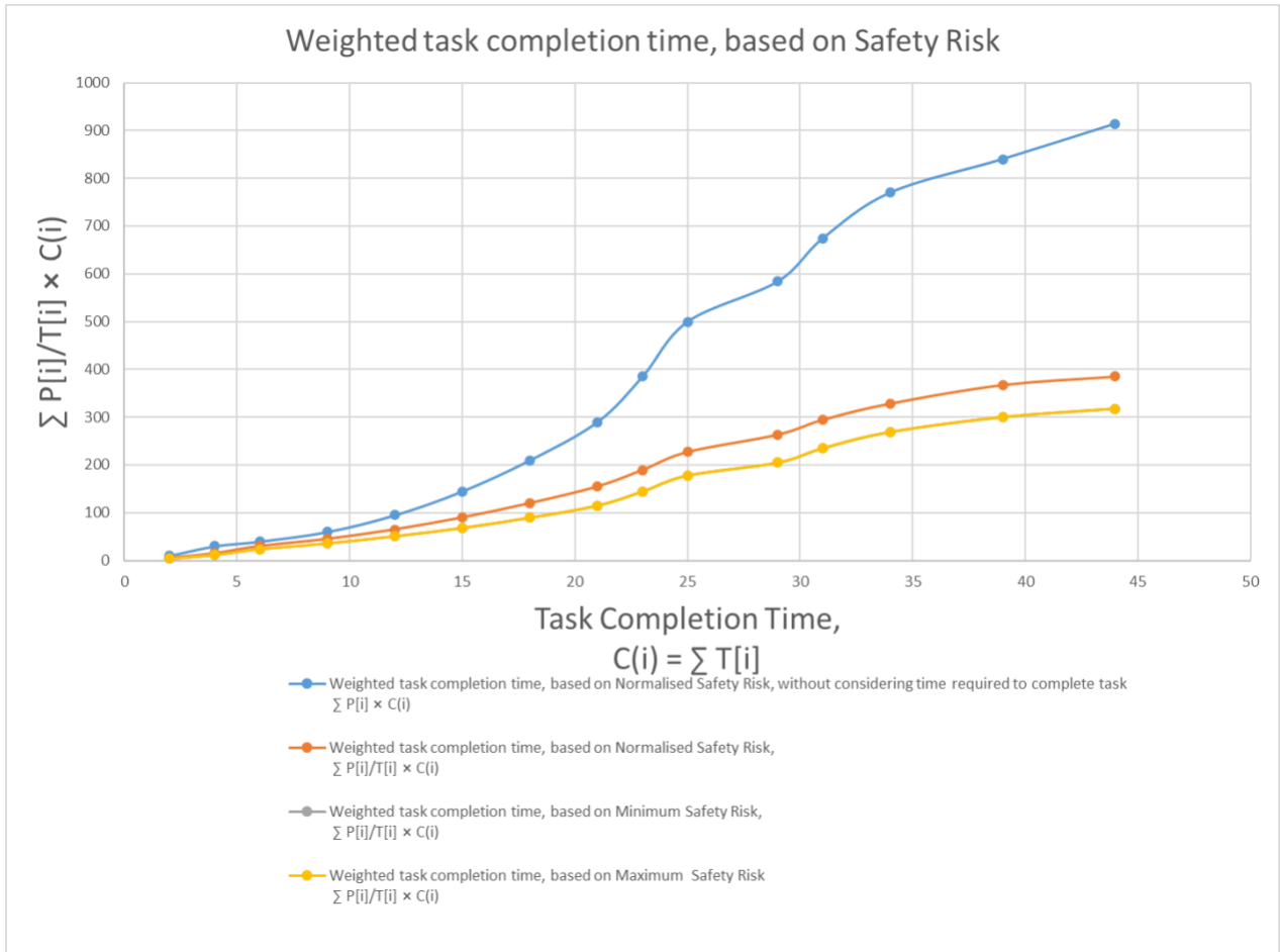
Figure 7: Weighted task completion time, based on Consequences of not doing the tasks – Safety Risk over Time required to complete task, \sum(P[i] / T[i]) \times C(i)
