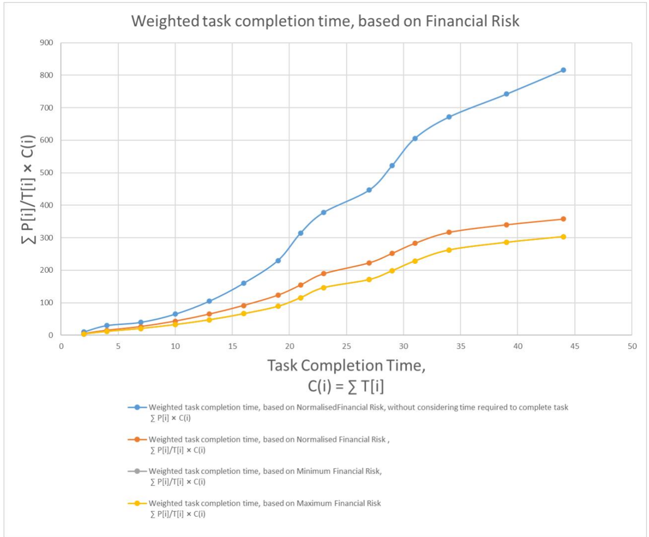
Figure 9: Weighted task completion time, based on Consequences of not doing the tasks – Financial Risk over Time required to complete task, \sum(P[i] / T[i]) \times C(i)
