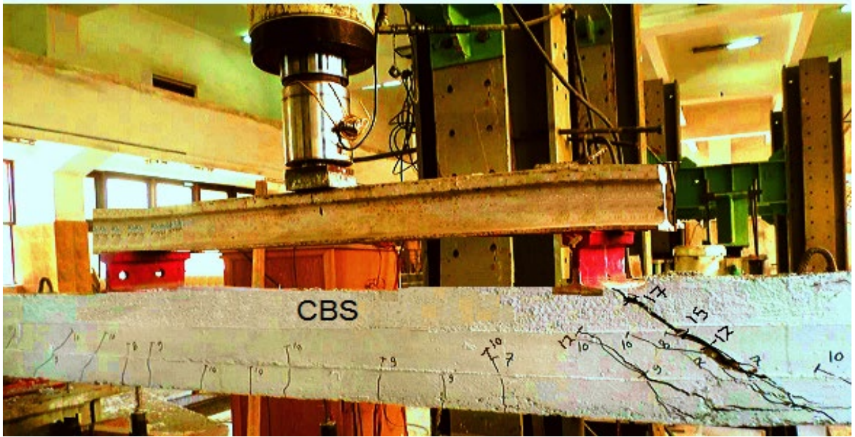
a) Control beam for shear
