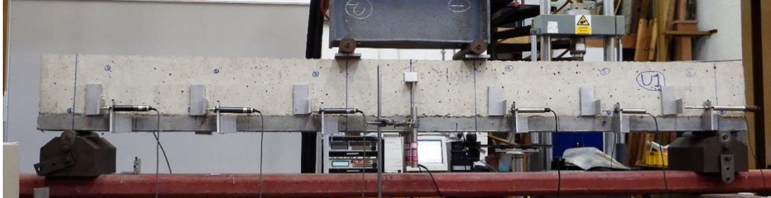
Figure 4 Experimental setup for the four point loading tests
