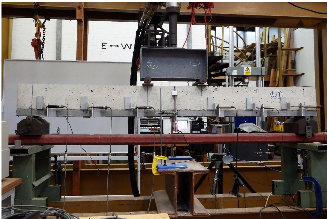
Figure 9 Experimental setup for the four point loading tests
