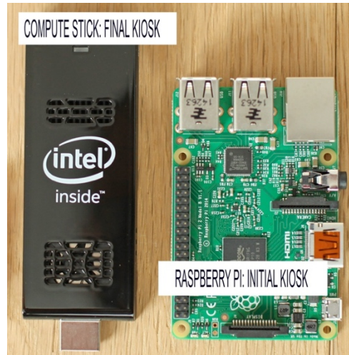
Figure 5.1 Size Comparison of Compute Stick against Raspberry Pi.
