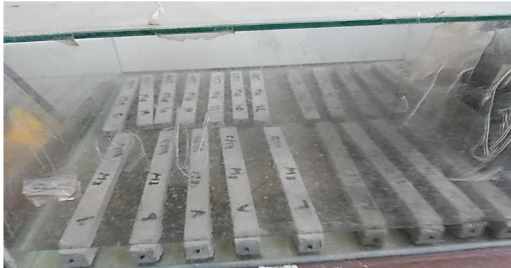
Fig. 10. Setup for sulfate attack test
