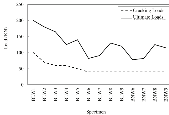
Fig. 5. Crack and ultimate load of tested deep beams.
