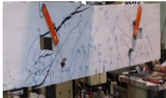
Fig. 18. Comparison between predicted and experimental crack pattern and failure modes for selected beams.
