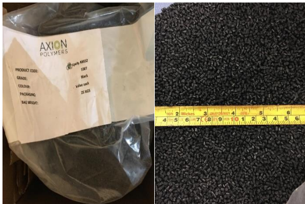
Fig. 3 Plastic Aggregate Material
