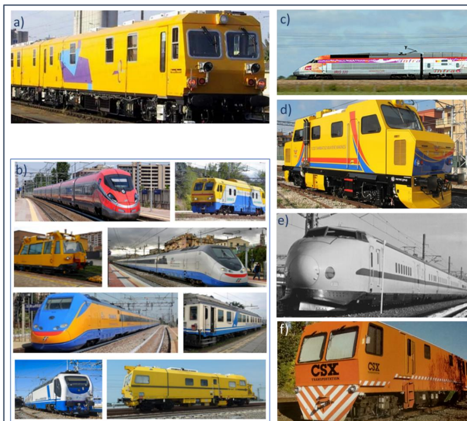
382 Fig. 4 a) UFM 160 (De Bold 2011), b) Diagnostic Trains Fleet of RFI (RFI 2018), c) Mauzin 383 synthétique IRIS 320 (Quiroga and Schnieder 2013), d) Automatic train examination stations (ATES) 384 (Artagan and Borecky 2015), Track Geometry Car for Shinkansen tracks (Miura et al. 1998), f) EM- 385 GMRS track car (Solomon 2001)
