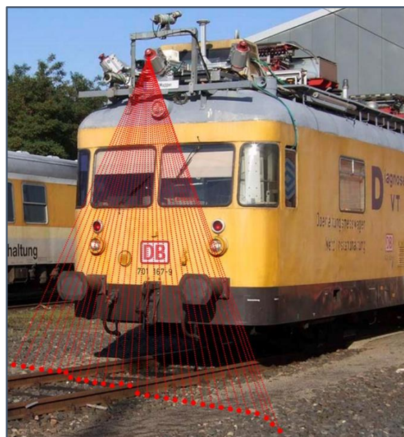
Fig. 7 An example of mobile mapping system mounted on a train with a number three laser scanners and
