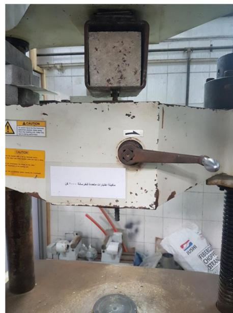
**Figure 8.** Pull Out Bond/Strength Test Setup.
