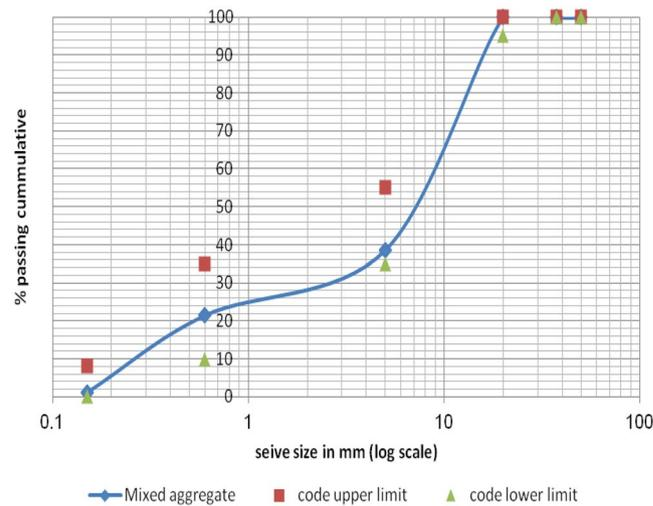
**Figure 3.** Mixed Aggregates Sieve Analysis According to Limits<sup>53</sup>.
