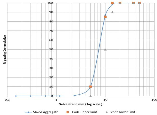
**Figure 2.** Dolomite Aggregates Sieve Analysis According to Limits<sup>53</sup>.
