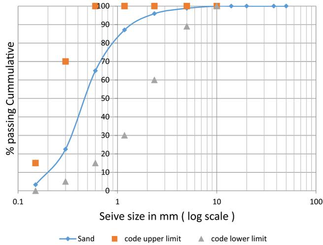
**Figure 1.** Fine Aggregates Sieve Analysis According to Limits<sup>53</sup>.
