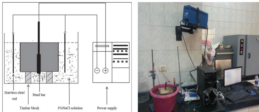
**Figure 7.** Corrosion or Electrochemical Test Set Up.
