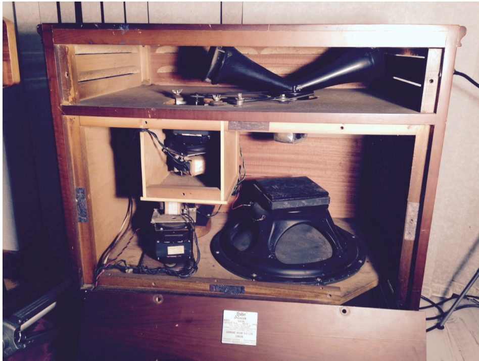
Figure 2.6 The Leslie speaker, showing the rotating speaker horns (top right). 45
