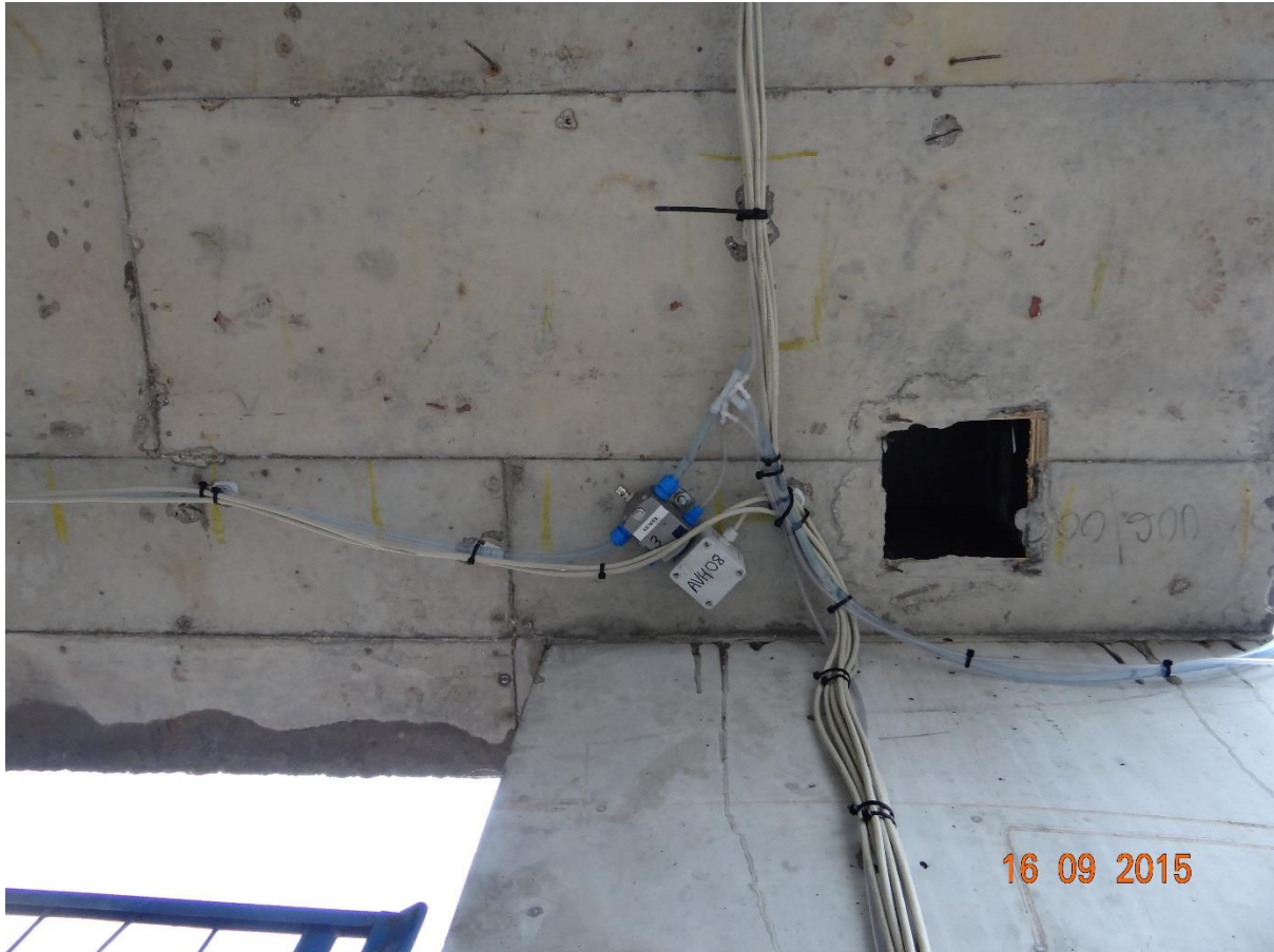
Figure 3.4 Hydrostatic Cells Levelling System Connected
