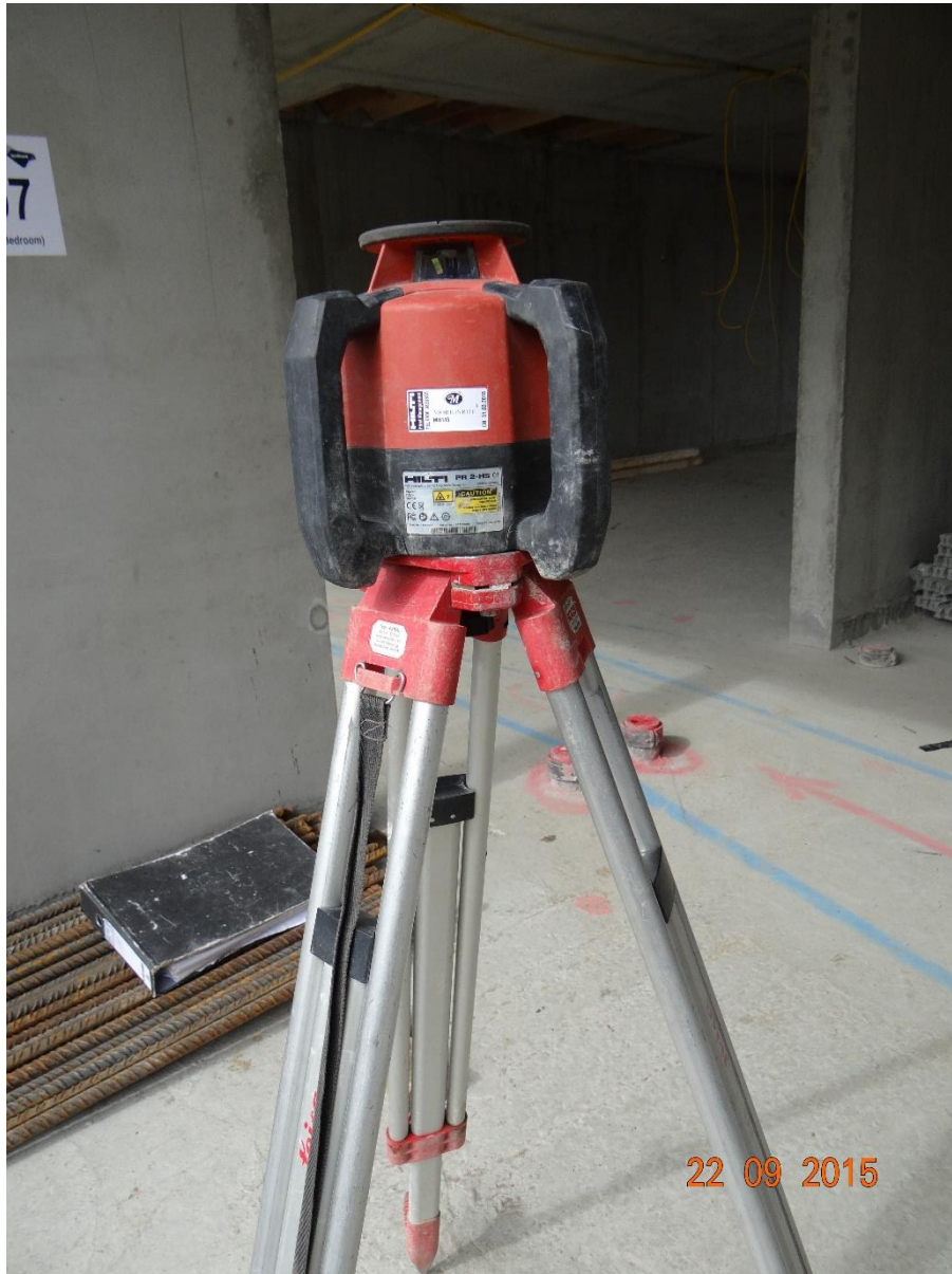
Figure 3.3 Level Observing Deflection on Slab
