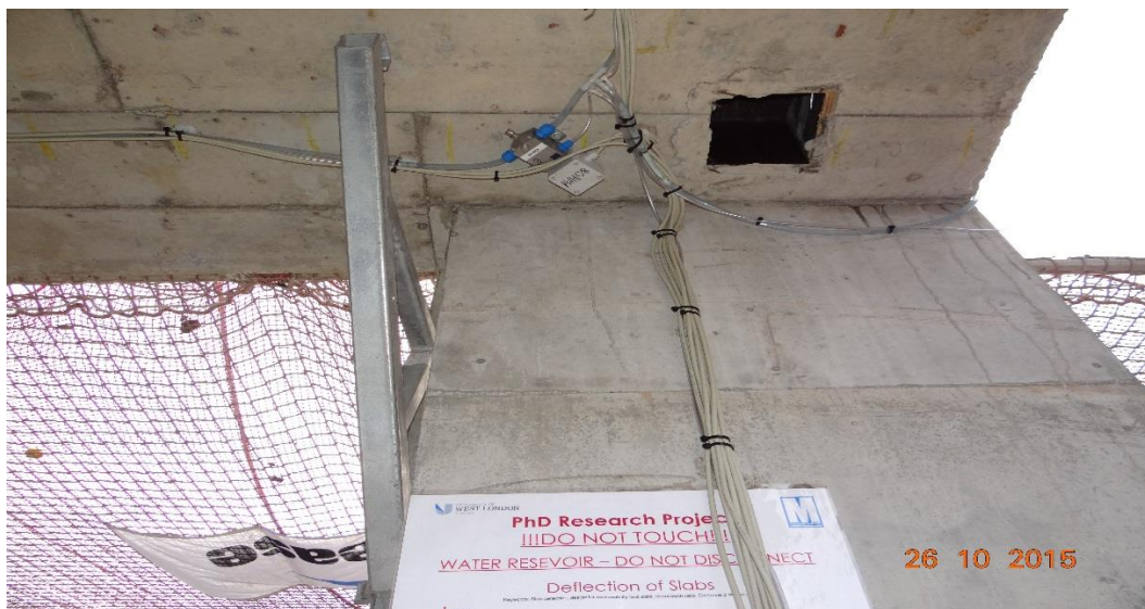
Figure 3.7 Hydraulic Cell Level Network Connection
