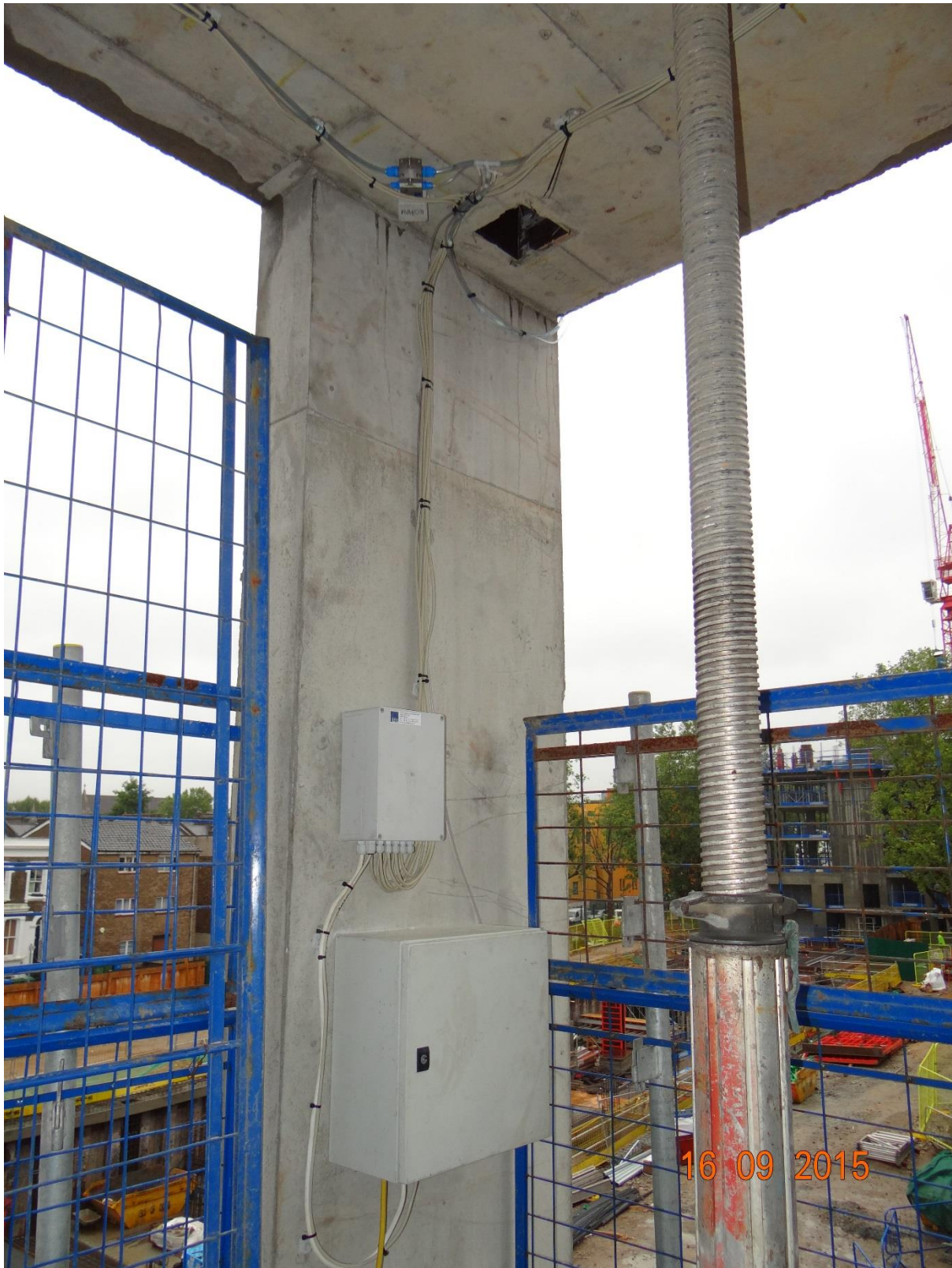
Figure 3.9 Hydrostatic Cells Levelling Connected to Data Box
