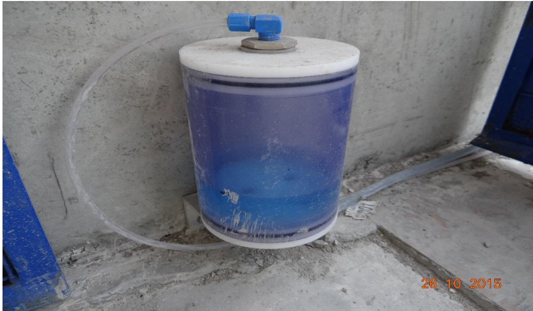
Figure 3.8 Hydraulic Cell Level water pressure reservoir
