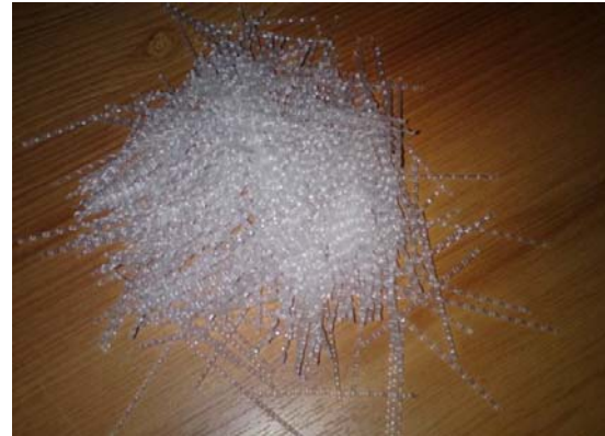
(a) HPP 45 fibre
