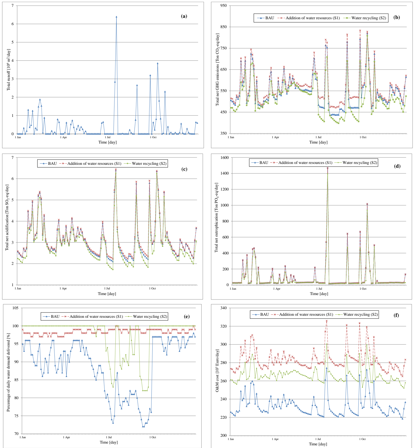
Fig. 10. Daily variations of the metrics for different strategies for (a) runoff (b) net GHG emissions (c) net acidification (d) net eutrophication, (e) water demand delivered, and (f) O&M cost.
