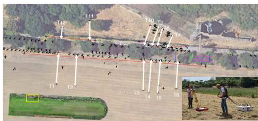
Figure 4. Position of the GPR scans acquired for the identification of the foundation level. The yellow box highlights the area of investigation
