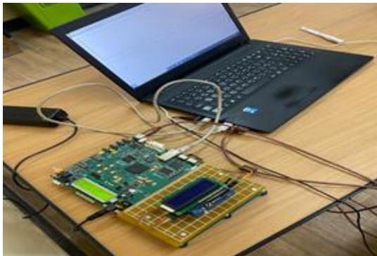
Figure. 17 HIL System Wiring
