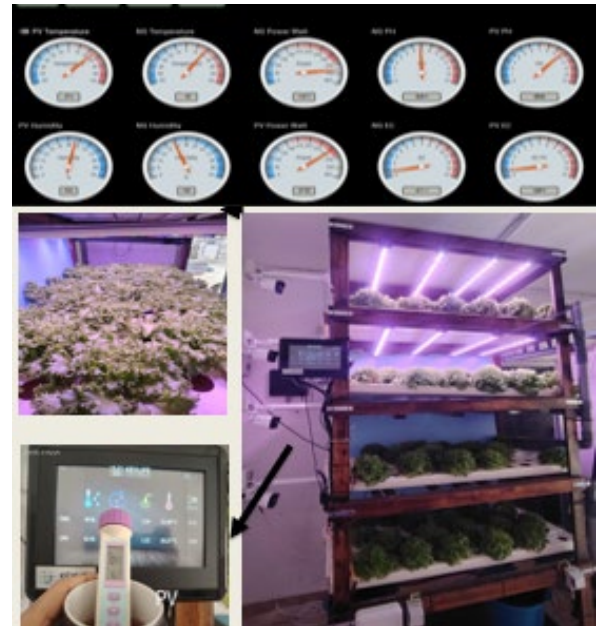
Fig. 1. CEA unit with IoT sensors (bottom 2 shelves are connected to the grid and top 2 to PV)
