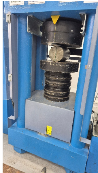
Figure 3. Split tension test setup.
