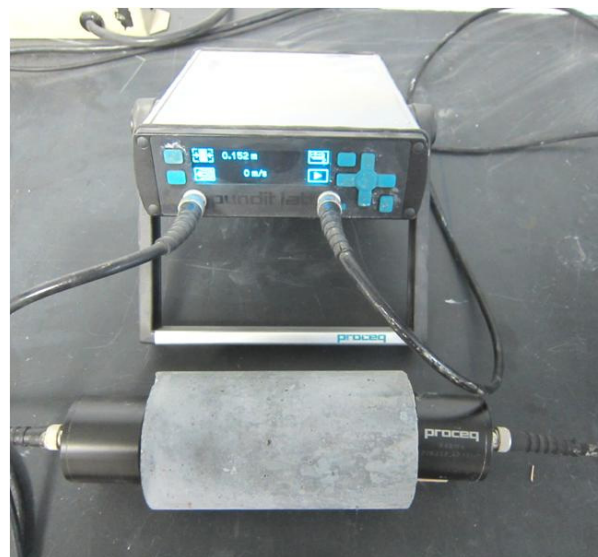
Figure 7. The ultrasound pulse velocity test setup.
