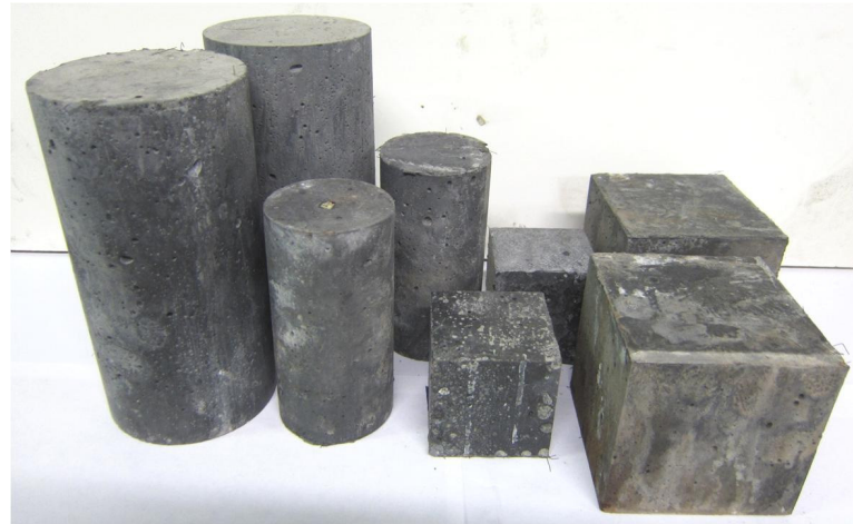
Figure 8. UHPC compression test specimens of different sizes and shapes.
