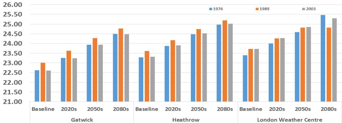
Figure 5.7 A comparison of average internal operative temperatures for Gatwick, Heathrow and London Weather Centre using UKCP09 1976, 1989 and 2003 medium 50% probabilistic weather data set scenarios with overheating analysis based on CIBSE TM52 adaptive thermal comfort criteria.
