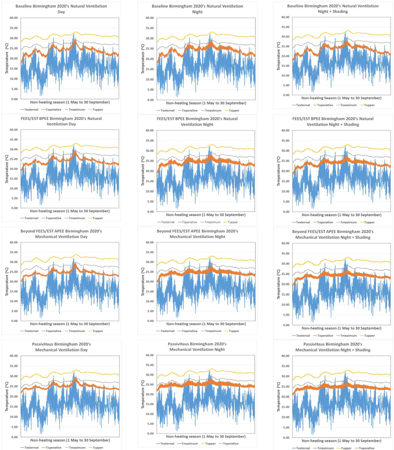
**Appendix 7.6 A comparison of whole building internal operative temperatures for Birmingham using CIBSE 2020's weather data set based on UKCIP02 climatic projections, varying ventilation scenarios and overheating analysis based on CIBSE TM52 adaptive thermal comfort criteria.**
