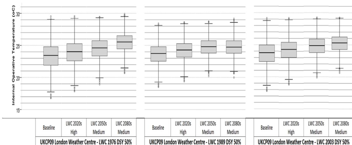
**Figure 5.12** Box and whiskers plot comparison of the internal operative temperatures reported in relation to the effect of the design summer year (DSY) medium 50% probabilistic scenarios of the 1976, 1989 and 2003 weather data sets of London Weather Centre
