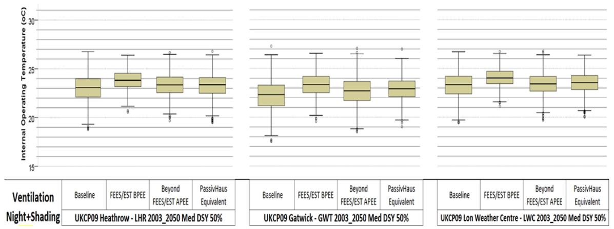
**Figure 8.6 Box and whiskers plots for night ventilation with shading scenario comparison of the internal operative temperatures effect of four standardized construction specifications based on 2003-2050 DSY Medium 50% probabilistic weather scenarios for Gatwick, Heathrow and London Weather Centre**
