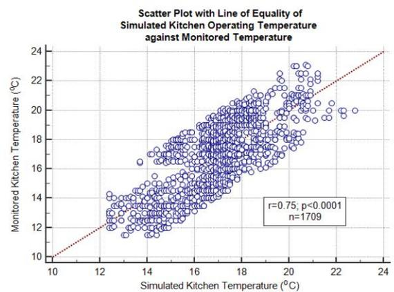
**Figure 4.4 Kitchen Operative temperatures Scatter plot with Line of Equality**
