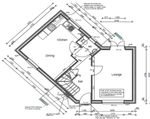
Figure 3.9 Architectural Ground Floor Plan
