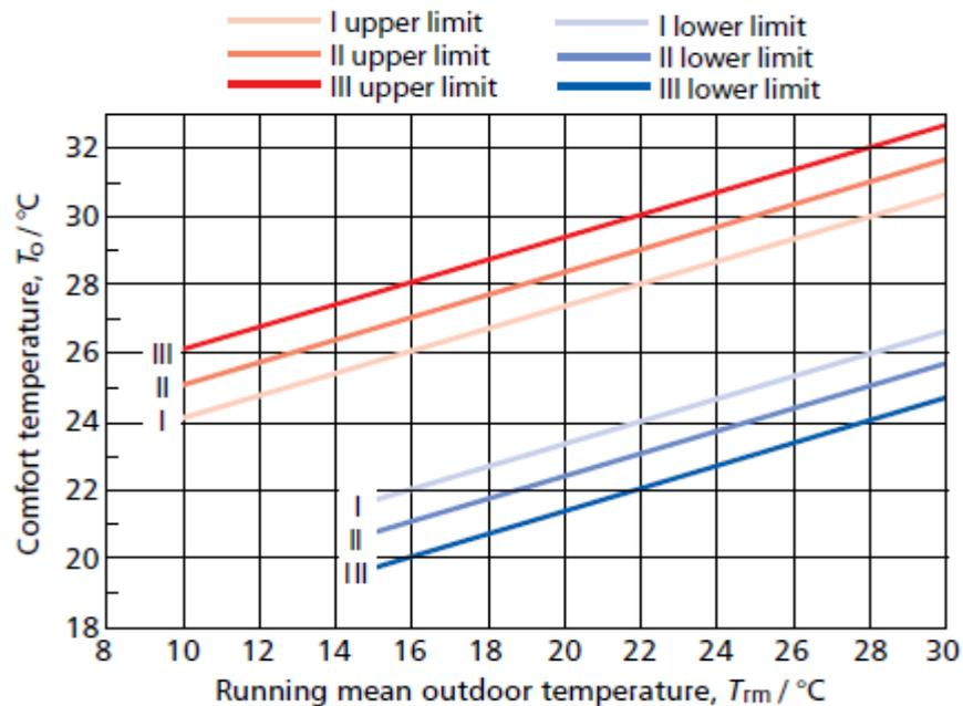
Figure 3.15 Limiting design values for the building operative temperature as against the exponentially weighted running mean of the external temperature. (Adapted from (BSI, 2007) and (CIBSE TM52))
