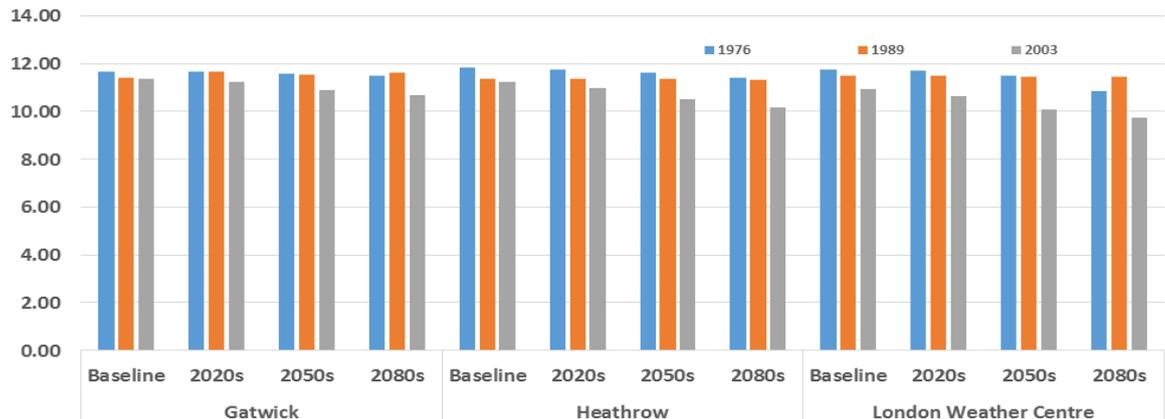
Figure 5.8 A comparison of the range internal operative temperatures for Gatwick, Heathrow and London Weather Centre using UKCP09 1976, 1989 and 2003 medium 50% probabilistic weather data set scenarios with overheating analysis based on CIBSE TM52 adaptive thermal comfort criteria.
