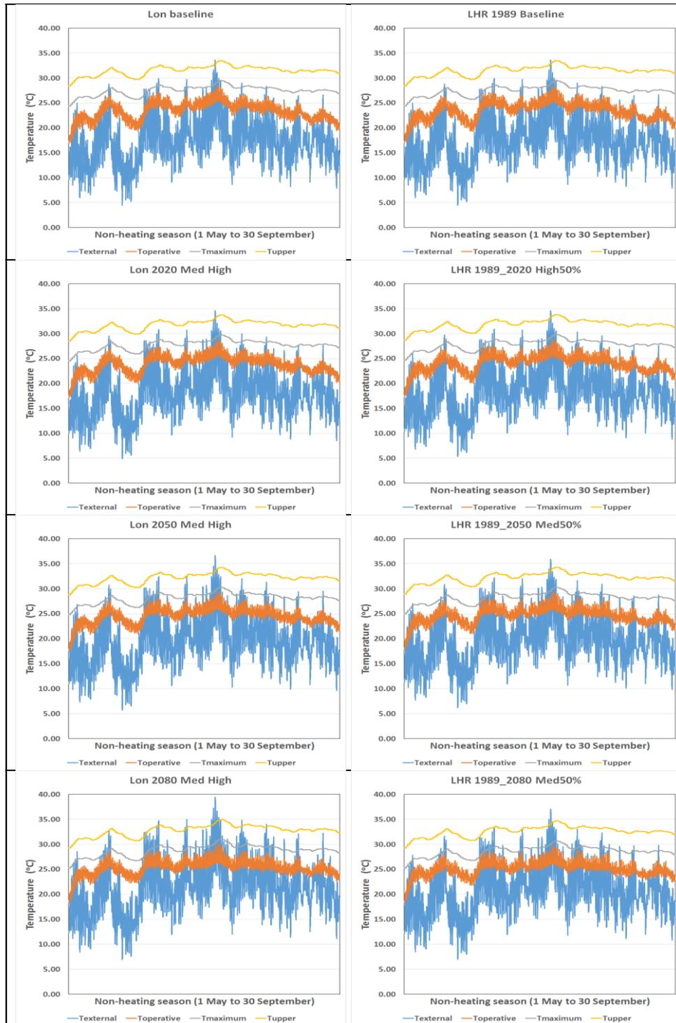
Appendix 5.1 A comparison of internal operative temperatures for UKCIP02 Heathrow DSY Medium High and UKCP09 Heathrow 1989 medium 50% probabilistic scenarios based on CIBSE TM52 adaptive thermal comfort criteria.
