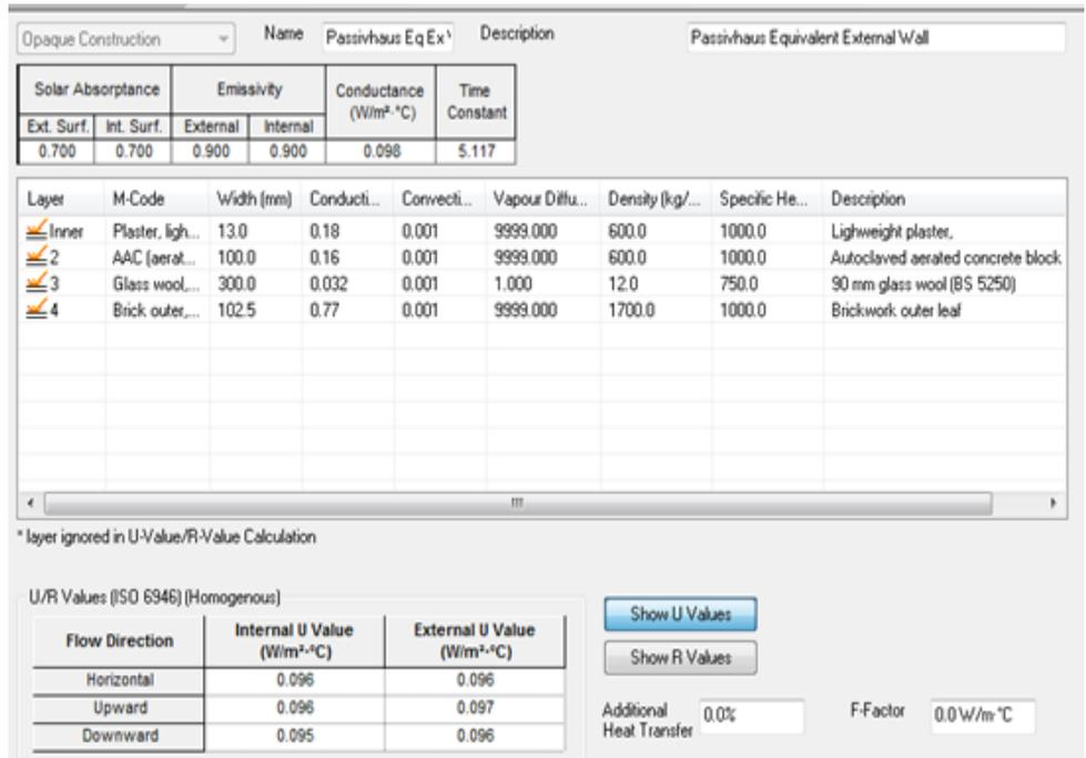
**Figure 3.14** Equivalent PassiHaus External Specification as designed for TAS
