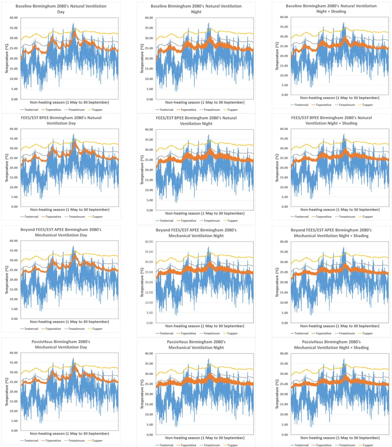
**Appendix 7.8 A comparison of whole building internal operative temperatures for Birmingham using CIBSE 2080's weather data set based on UKCIP02 climatic projections, varying ventilation scenarios and overheating analysis based on CIBSE TM52 adaptive thermal comfort criteria.**
