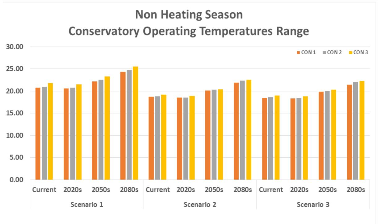
Senario 1- No shading, Cross day ventilation in all direction, Openable window proportion 100%; at least 5% of total floor area.
