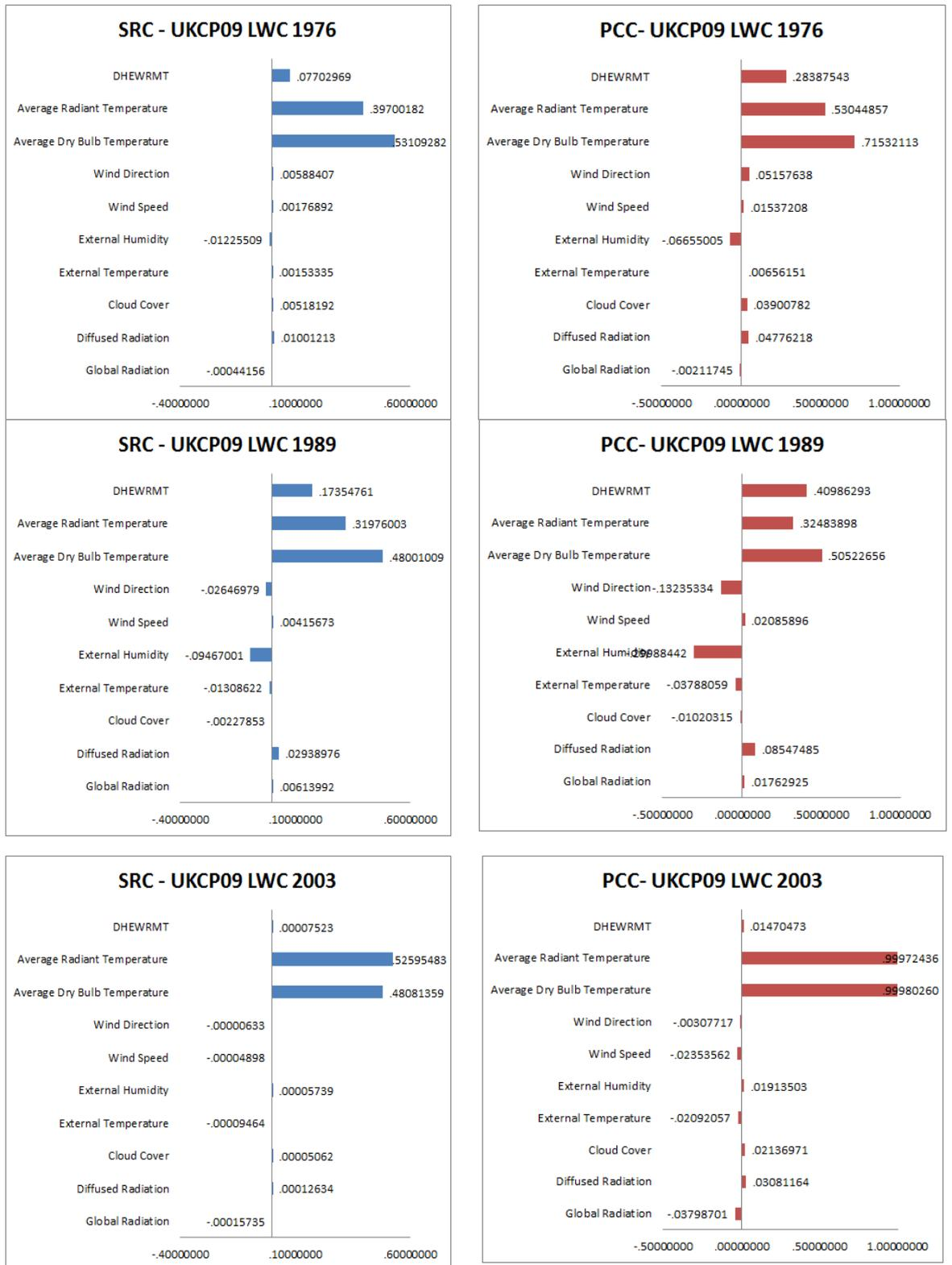
**Figure 5.17 Comparison of the standardized regression coefficient (SRC) and the partial correlation coefficients (PCC) of the weather input variables for the UKCP09 1976, 1989 and 2003 London Weather Centre weather data sets.**
