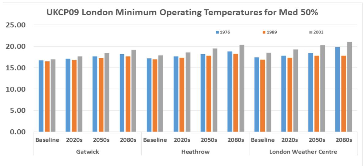
**Figure 5.6 A comparison of minimum internal operative temperatures for Gatwick, Heathrow and London Weather Centre using UKCP09 1976, 1989 and 2003 medium 50% probabilistic weather data set scenarios with overheating analysis based on CIBSE TM52 adaptive thermal comfort criteria.**
