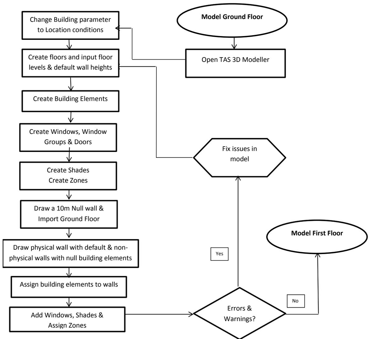
**Figure 3.4 Ground floor modelling process**
