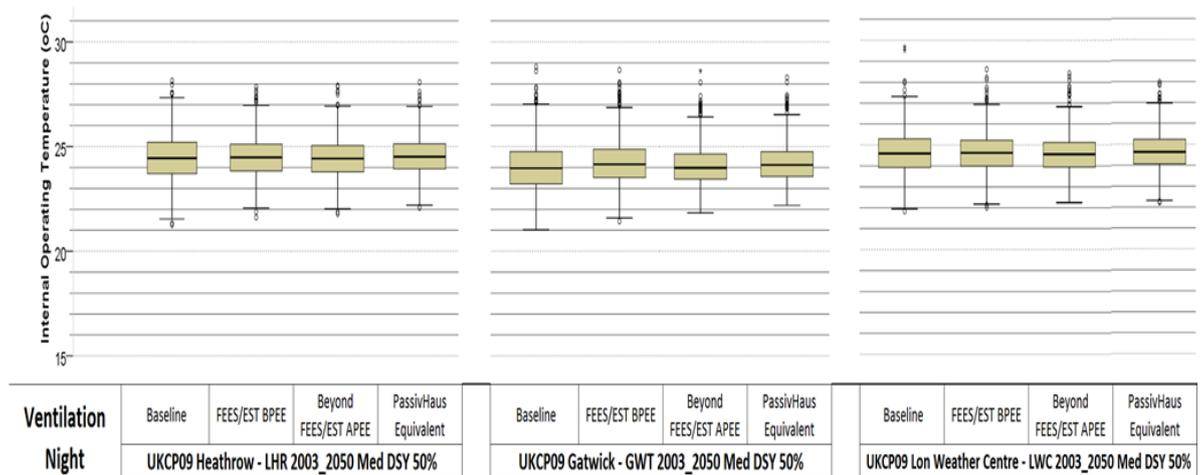
**Figure 8.5 Box and whiskers plots for night ventilation scenario comparison of the internal operative temperatures effect of four standardized construction specifications based on 2003-2050 DSY Medium 50% probabilistic weather scenarios for Gatwick, Heathrow and London Weather Centre**
