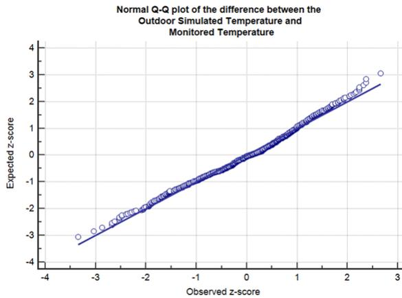
**Figure 4.7 Normal Q-Q plot of the difference between Outdoor Simulated and Monitored Temperatures**
