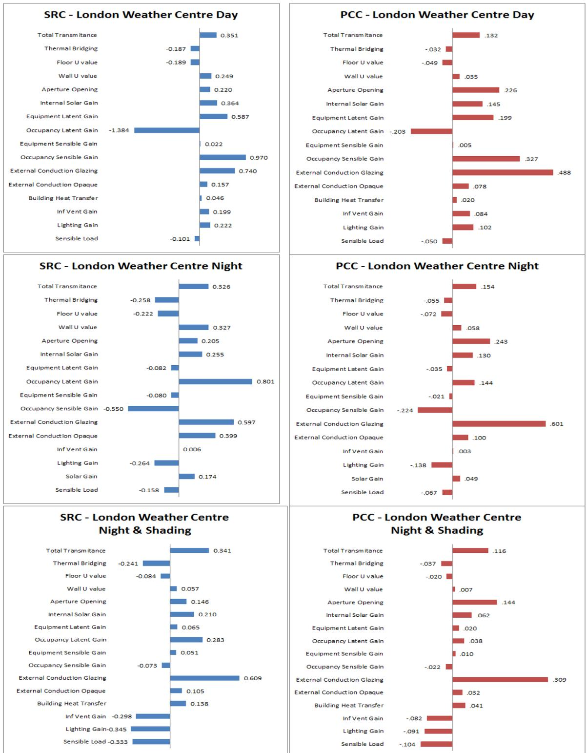
Figure 8.12 Comparison of the standardized regression coefficient (SRC) and the partial correlation coefficients (PCC) of the future building adaptation measures input variables for the standardized construction specifications based on UKCP09 LWC 2003-2050 Med 50% weather data for London Weather Centre under day, night and night with shading ventilation scenarios.
