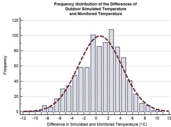
**Figure 4.5** Frequency distribution of Outdoor Simulated and Monitored Temperatures
