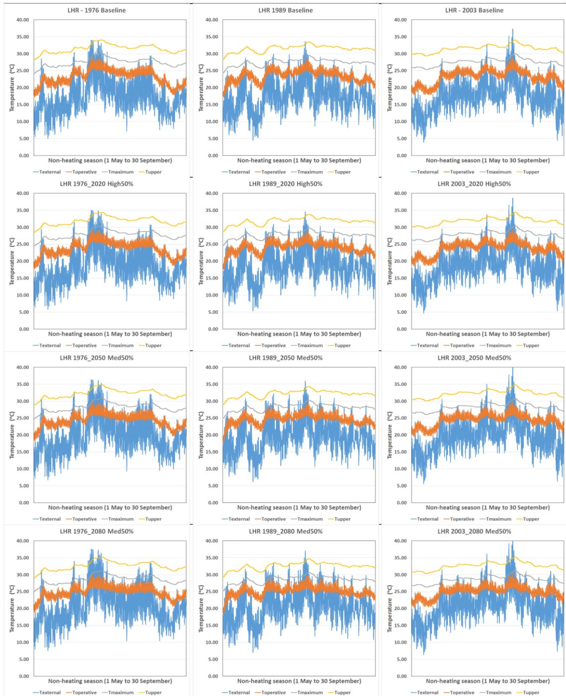
**Appendix 5.2 A comparison of internal operative temperatures for Heathrow using UKCP09 1976, 1989 and 2003 medium 50% probabilistic weather data set scenarios with overheating analysis based on CIBSE TM52 adaptive thermal comfort criteria.**
