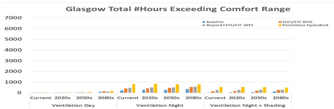
**Figure 7.1 A comparison of internal operative temperatures total number of hours exceeding comfort range analysis of respective zone results for London, Birmingham and Glasgow respectively based on CIBSE TM52 adaptive thermal comfort criteria.**
