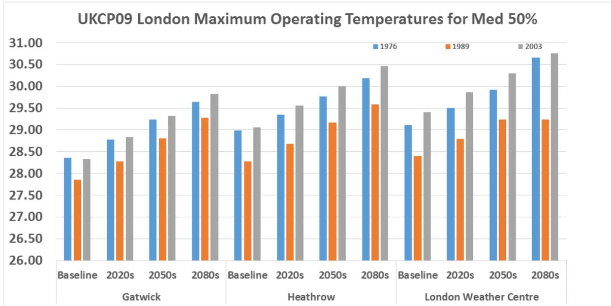
**Figure 5.5 A comparison of maximum internal operative temperatures for Gatwick, Heathrow and London Weather Centre using UKCP09 1976, 1989 and 2003 medium 50% probabilistic weather data set scenarios with overheating analysis based on CIBSE TM52 adaptive thermal comfort criteria.**
