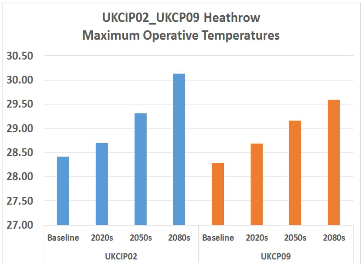
Figure 5.1 Maximum operative temperatures for UKCIP02 Heathrow DSY Medium High and UKCIP09 Heathrow 1989 medium 50% probabilistic scenarios
