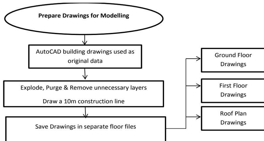
**Figure 3.3 Prepare Drawings for Modelling**
