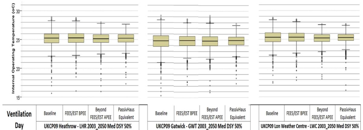
**Figure 8.4** Box and whiskers plots for day ventilation scenario comparison of the internal operative temperatures effect of four standardized construction specifications based on 2003-2050 DSY Medium 50% probabilistic weather scenarios for Gatwick, Heathrow and London Weather Centre
