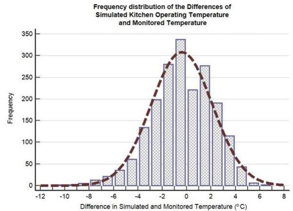
**Figure 4.6** Frequency distribution of Kitchen Simulated and Monitored Temperatures
