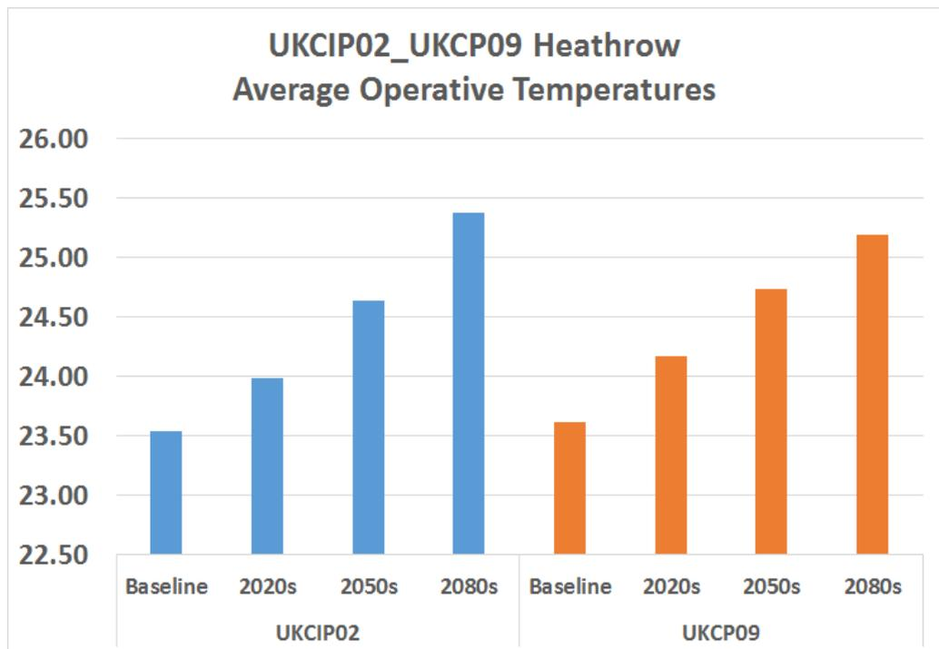
**Figure 5.3 Average operative temperatures for UKCIP02 Heathrow DSY Medium High and UKCP09 Heathrow 1989 medium 50% probabilistic scenarios**
