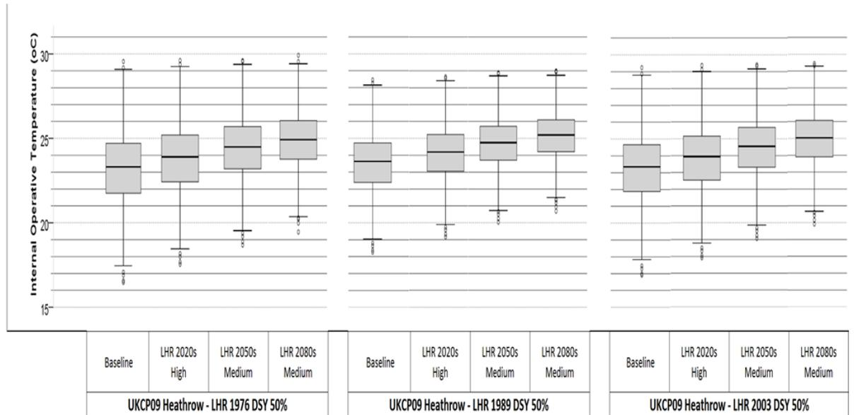
**Figure 5.11 Box and whiskers plot comparison of the internal operative temperatures reported in relation to the effect of the design summer year (DSY) medium 50% probabilistic scenarios of the 1976, 1989 and 2003 weather data sets of Heathrow**
