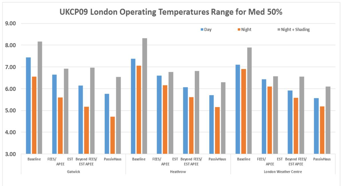
**Figure 8.4 Range operative temperatures for UKCP09 Gatwick, Heathrow and London Weather Centre 2003\_2050 Medium DSY 50% probabilistic scenarios**
