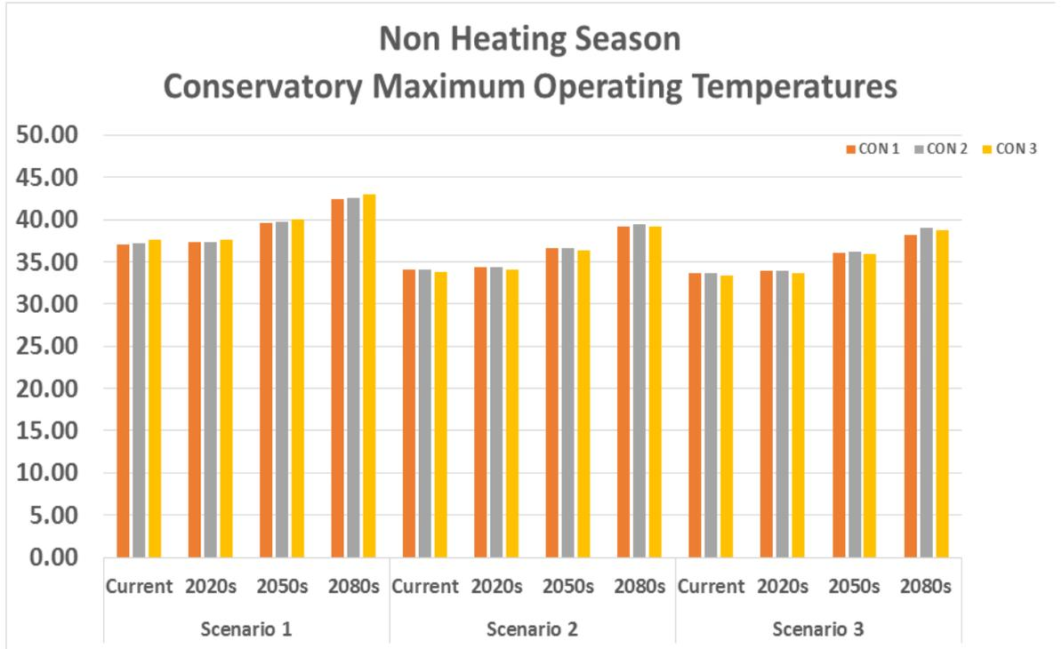
Scenario 1- No shading, Cross day ventilation in all direction, Openable window proportion 100%; at least 5% of total floor area.
