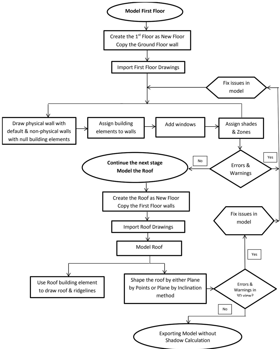
**Figure 3.5 First floor/Roof modelling process**
