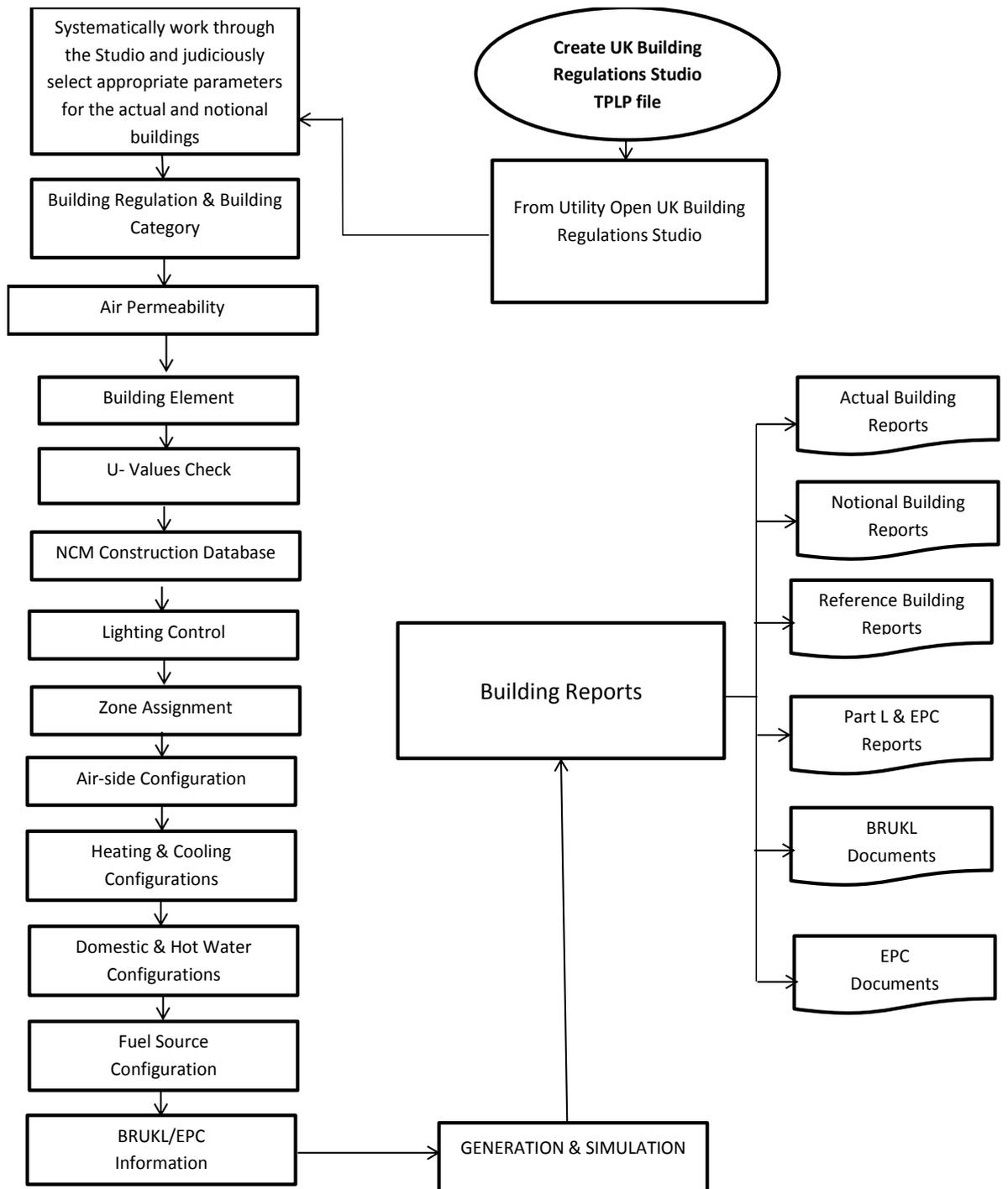
**Figure 3.7 UK Building Regulation Studio Simulation process**
