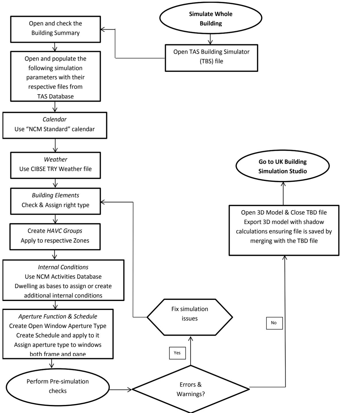
Figure 3.6 Thermal Simulation process
