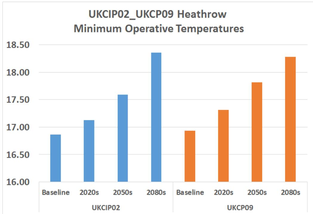
**Fig 5.2 Minimum operative temperatures for UKCIP02 Heathrow DSY Medium High and UKCP09 Heathrow 1989 medium 50% probabilistic scenarios**
