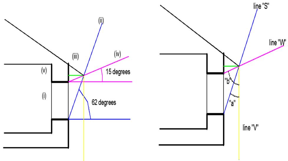
**Figure 3.17 Sizing of overhang/awnings adapted from EREC 2000 and BRE 1988**
