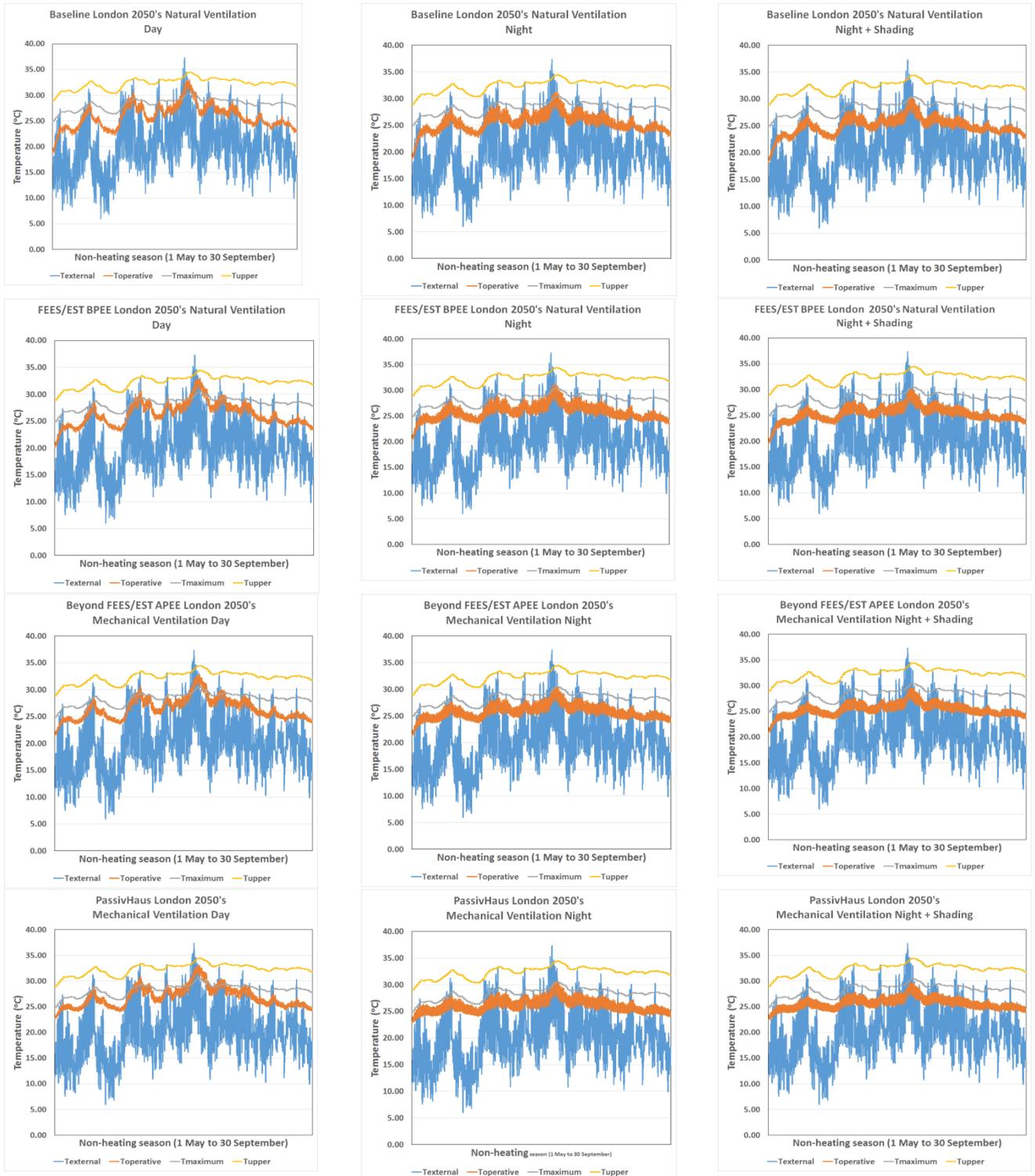
**Appendix 7.3 A comparison of whole building internal operative temperatures for London using CIBSE 2050's weather data set based on UKCIP02 climatic projections, varying ventilation scenarios and overheating analysis based on CIBSE TM52 adaptive thermal comfort criteria.**
