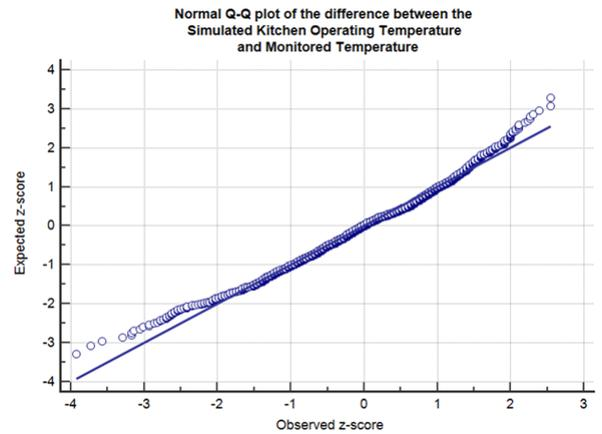
**Figure 4.8 Normal Q-Q plot of the difference between Kitchen Simulated and Monitored Temperatures**
