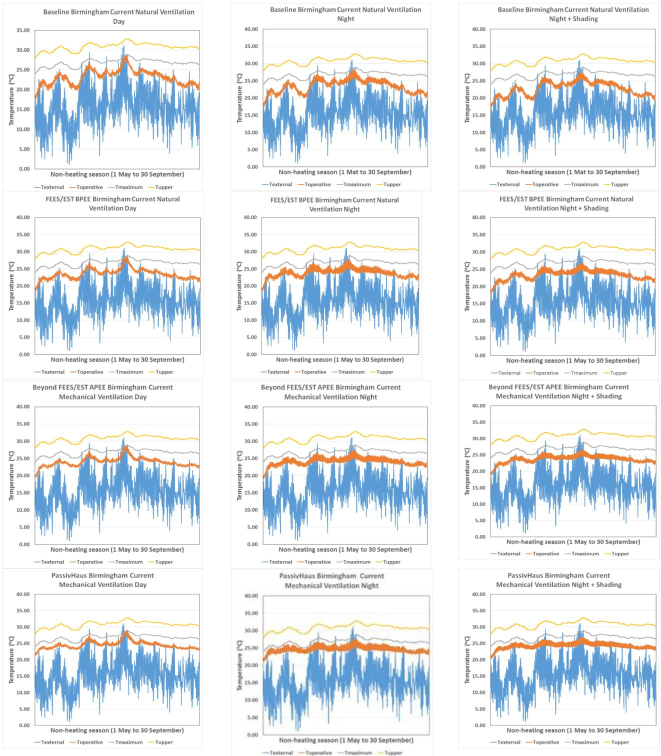
**Appendix 7.5 A comparison of whole building internal operative temperatures for Birmingham using CIBSE current weather data set based on UKCIP02 climatic projections, varying ventilation scenarios and overheating analysis based on CIBSE TM52 adaptive thermal comfort criteria.**
