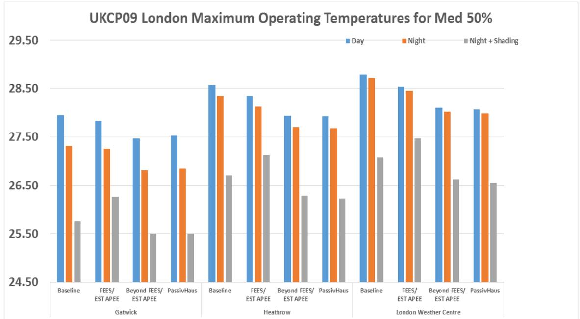
Figure 8.1 Maximum operative temperatures for UKCP09 Gatwick, Heathrow and London Weather Centre 2003\_2050 Medium DSY 50% probabilistic scenarios
