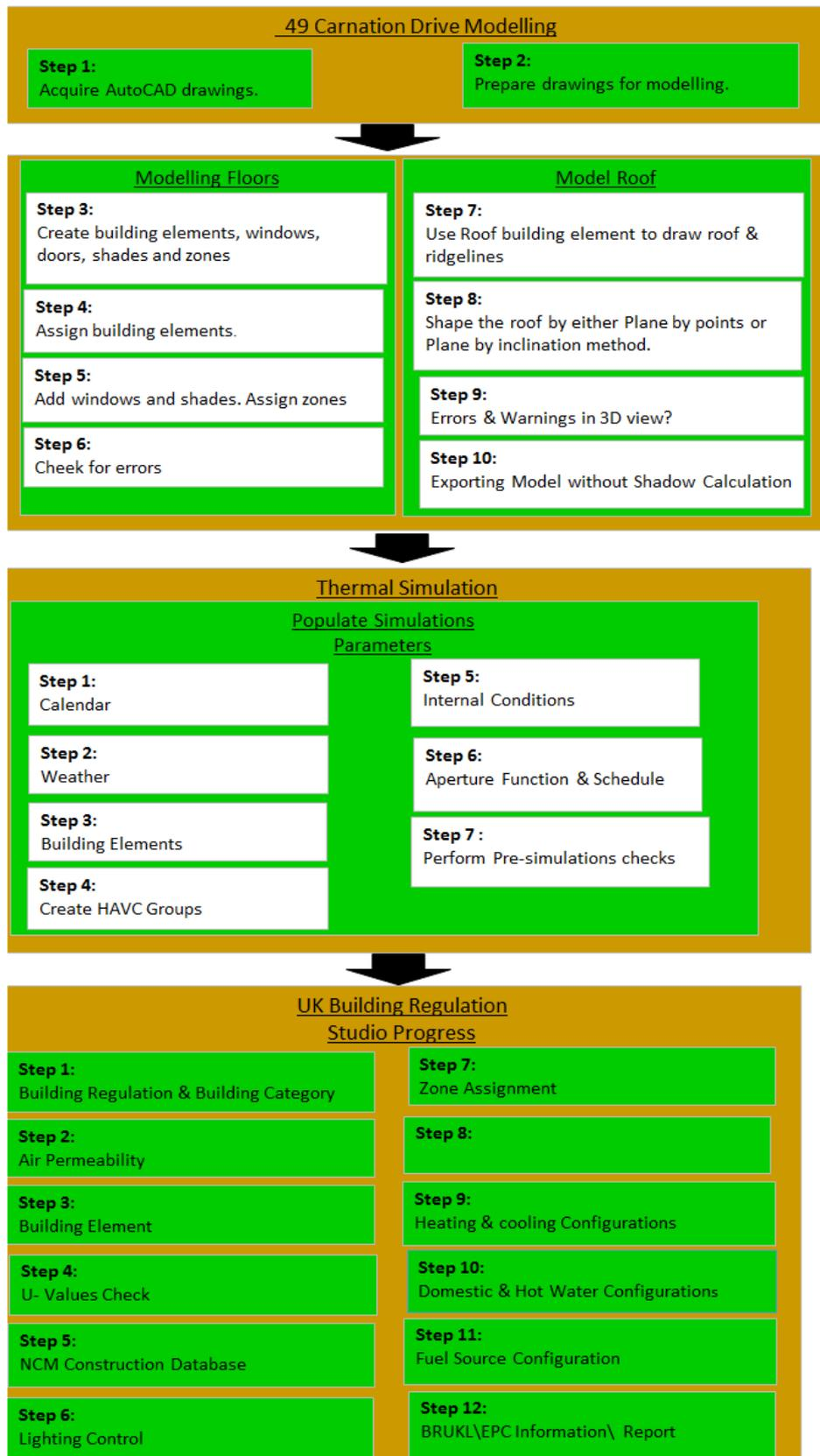
**Figure 3.16 Methodological processes for modelling and simulating detached dwelling with attached conservatory thermal performance.**
