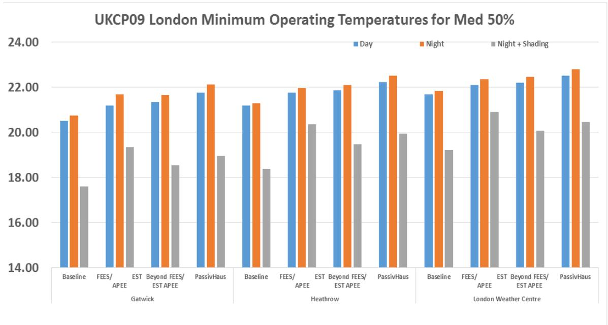
Figure 8.2 Minimum operative temperatures for UKCP09 Gatwick, Heathrow and London Weather Centre 2003\_2050 Medium DSY 50% probabilistic scenarios
