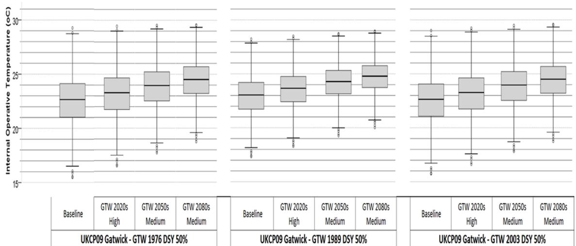
**Figure 5.10 Box and whiskers plot comparison of the internal operative temperatures reported in relation to the effect of the design summer year (DSY) medium 50% probabilistic scenarios of the 1976, 1989 and 2003 weather data sets of Gatwick**
