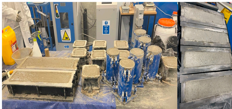
Figure 4. Casted set of concrete specimens.
