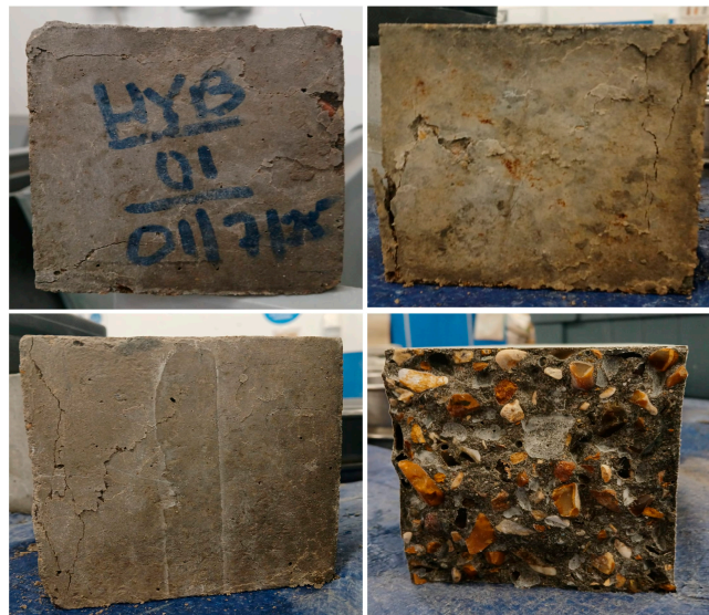
Figure 12. Ductile failure of hybrid mix concrete.
