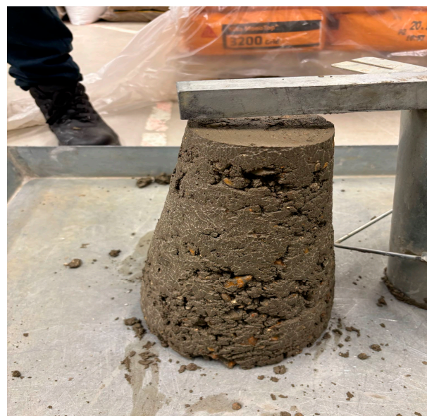
Figure 8. Reduction in slump due to balling effect.
