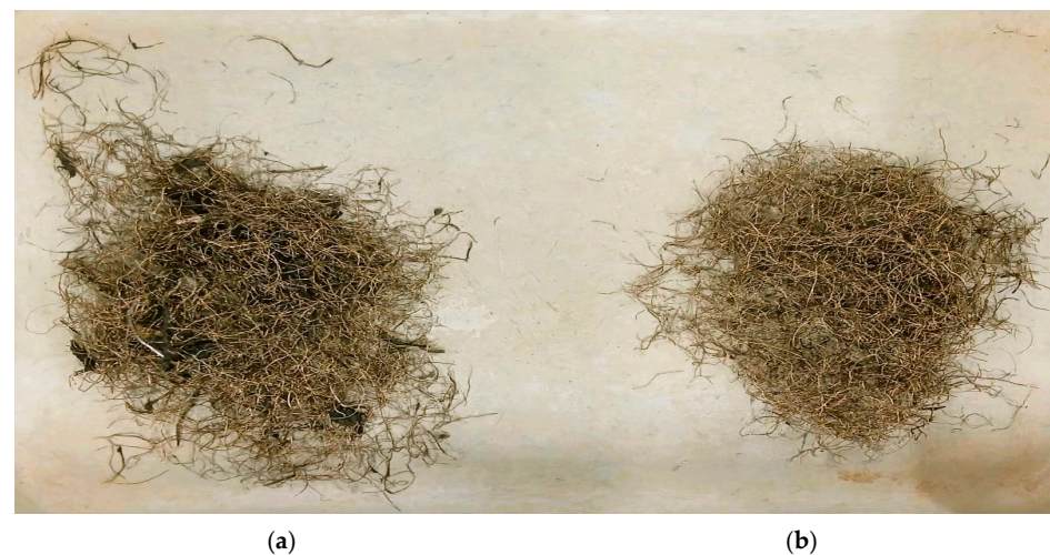
Figure 2. (a) RTSF with impurities; (b) RTSF after impurity removal.
