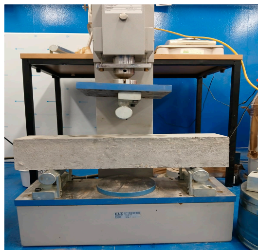
Figure 15. Flexural strength test arrangement.
