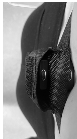
Figure 3. The stacking position of the accelerometers during the controlled activities and daily living conditions in part 1.
