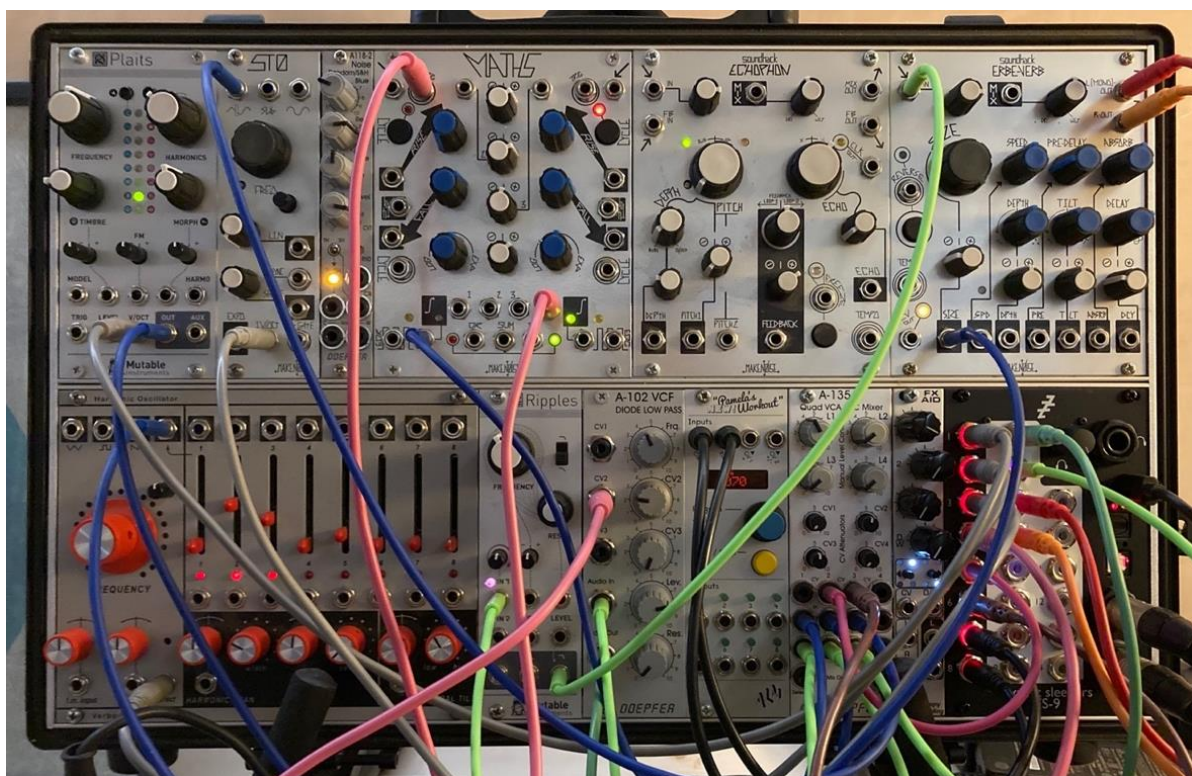
Figure 4-2 – An early version of the system, featuring MIDI-to-CV conversion via the Expert Sleepers ES9.
