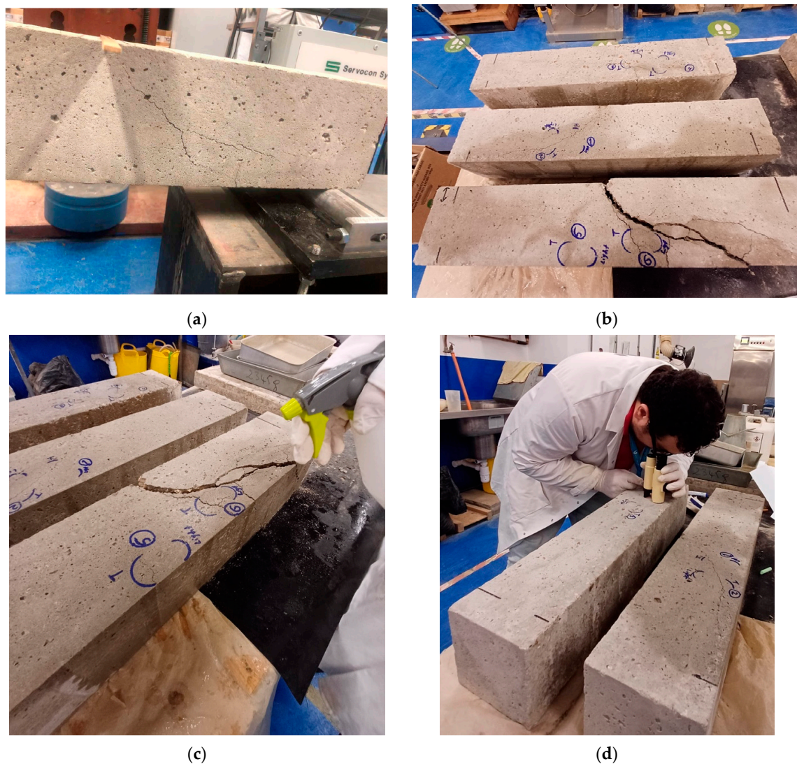
Figure 7. Application of enzymatic self-healing: (a) Controlled cracking of beams, (b) Concrete beams with various crack sizes, (c) Spraying the concrete beams with self-healing solution, (d) Measuring the healing potential using a microscope.
