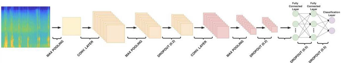
Fig. 2. The CNN structure applied in Cough Detection System.
