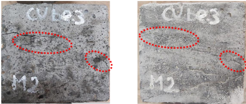
Figure 17. Self-Healing Concrete Samples (Shaaban et. al 2023)
