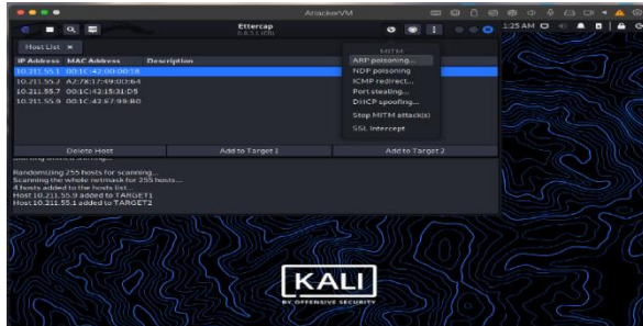
Fig 2. Adding the Target Device to Ettercap
