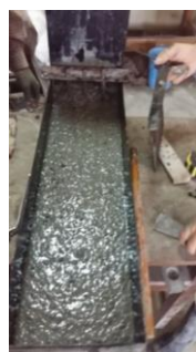
(a) Slump flow and L box for mix containing 10% MK (M3) (accepted as SCC)
