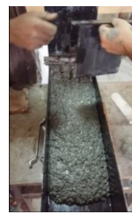
(b) Slump flow and L box for mix containing 15% MK (failed as SCC)
