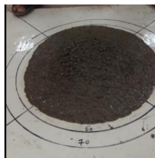
(b) Slump flow and L box for mix containing 15% MK (failed as SCC)
