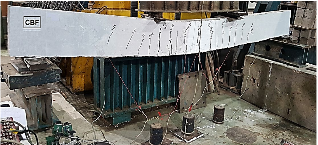
h) Control beam for flexure
