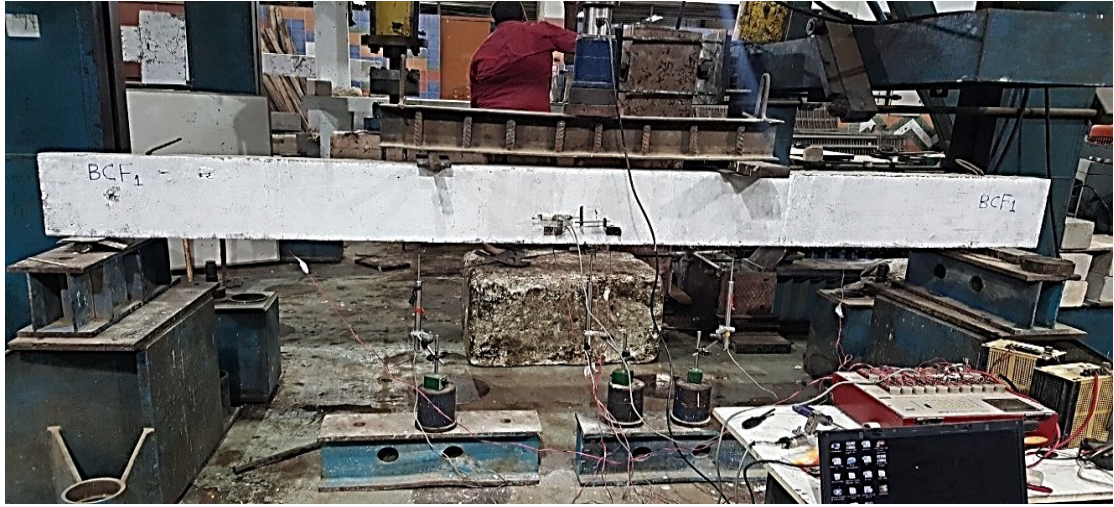
a) Beam specimen strengthened for flexure
