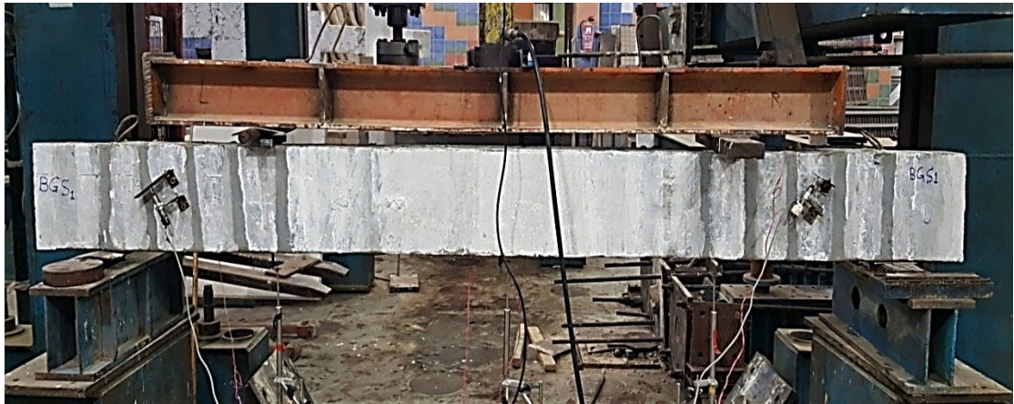
b) Beam specimen strengthened for shear
