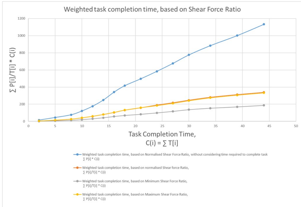
Figure 4.10: Weighted task completion time, based on operating conditions – Strength, Shear Force Ratio over Time required to complete task, \sum P[i] / T[i] * C(i)
