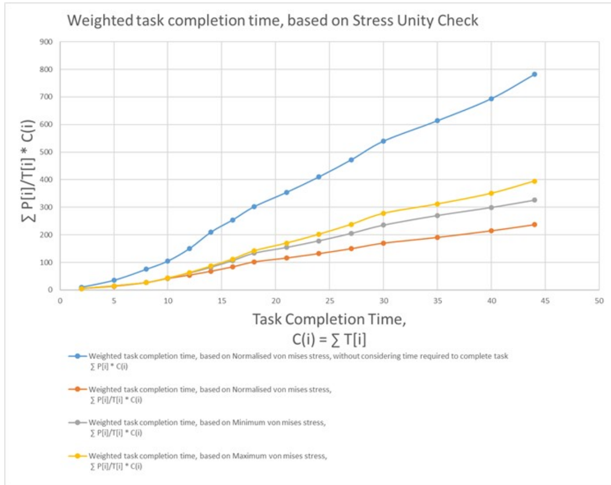
Figure 4.4: Weighted task completion time, based on design feature - Stress Unity Check over Time required to complete task, \sum P[i] / T[i] * C(i)
