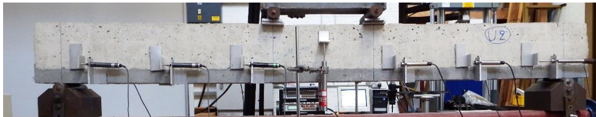
Figure 5 Experimental setup for the testing of beams
