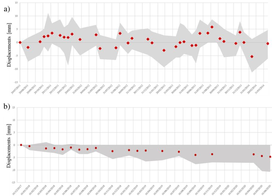
**Fig. 3.** PSI time-series and deformation velocity from: a) PS samples related to the COSMO-SkyMed, (©ASI –2011-2014)- PST-A project; b). PS time-series of the TerraSAR-X Products (© DLR-German Aerospace Agency).SAR images provided by ESA
