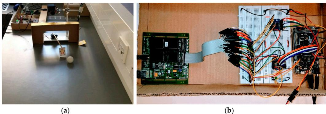
**Figure 6.** (a) Setup of the neuromorphic robotic goalkeeper. (b) Connections between the modules. One input/output port is used on SpiNNaker (SpiNN-3) board (shown left) and set in SpiNNakerLink class. Two chips on the protoboard are level shifters (1.8 V to/from 3.3 V), which are used between the microcontroller and SpiNNaker. The microcontroller (Arduino Due) is at the right end of the picture.
