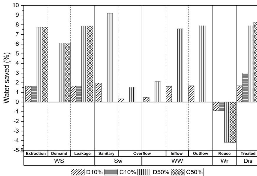
**Fig. 2. The proportion of water saved per subsystem component**
