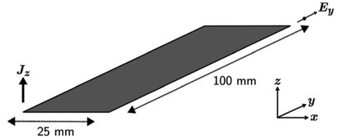
Fig. 3.  $z$ -directed Hertzian dipole over a PEC plate. The spatial step is  $\Delta x = \Delta y = \Delta z = 1$  mm, and the time-step is 0.99 times the Courant limit. The thickness of the PML equals  $d = 10$  mm.  $E_y$  is monitored in the opposite corner of the source's location, one Yee cell away from the PEC plate [6].
