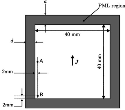
Fig. 1.  $y$ -directed current source is located at the center of a  $40 \times 40 TE_z$  FDTD grid. The electric field  $E_y$  is probed at  $A$  and  $B$  points. The spatial step is  $\Delta x = \Delta y = 1$  mm, and the time-step is 0.99 times the Courant limit. The thickness of the PML equals  $d = 10$  mm [6].
