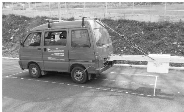
Figure A.5: GPR survey van mounting the air-launched antenna RIS Hi-Pave HR1 1000, manufactured by IDS Ingegneria dei Sistemi S.p.A., Italy.
