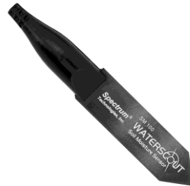
Figure 3.2: Capacitance probe WaterScout SM100, manufactured by Spectrum Technologies, Inc., USA.
