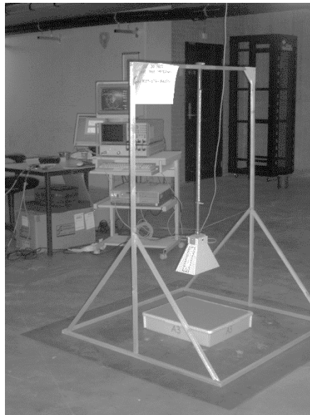
Figure A.6: SFCW radar set-up using a vector network analyzer HP 8573C (manufactured by Hewlett Packard Company, USA) and a linear polarized double-ridged broadband TEM horn BBHA 9120 A (manufactured by Schwarzbeck Mess-Elektronik, Germany), in a mono-static configuration.
