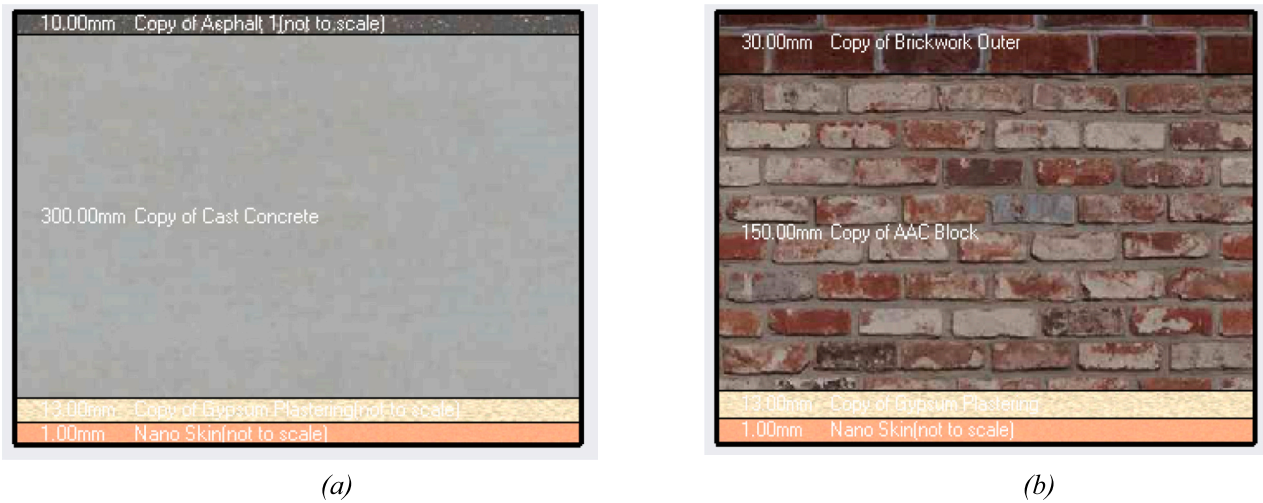
Fig. 9. (a) Detail of the roof with a layer of nano paint and (b) detail of external wall materials with a layer of Nano paint.
