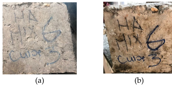
Fig.2 Typical cube specimen (a) after pre-damaged by 60 to 85 % of the ultimate capacity after healing process exposure, and (b) testing the pre-damaged specimens till crushing failure.
