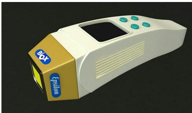
Fig. 12. The Epsilon futuristic concept with moving head, screen, and functional buttons
