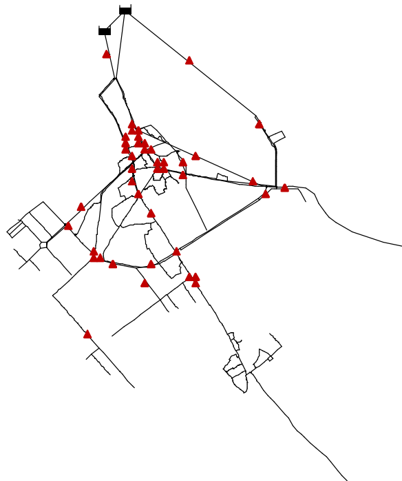
Figure 4. Potential locations for PRV installation
