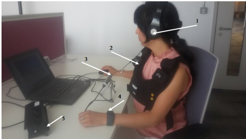
Fig. 1. Experimental setup. The users were wearing: (1) i-shine headphone, (2) the KOR-FX haptic vest, their eye gaze was captured with (3) the EyeTribe eye tracker, while their heart rate was measured with (4) Mio Link; olfactory effects were diffused using Exhalia (5).
