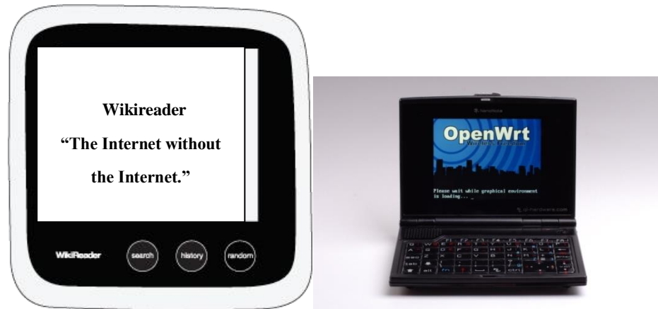
Figure 1a. Wikireader – offline handheld reading device. Figure 1b. Ben Nanonote - an ultra-small form factor copyleft computing device which has 336 MHz XBurst CPU, 3.0” display and 2GB NAND flash memory.
