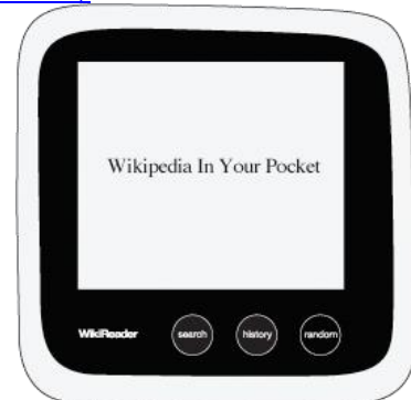
figure 2. Wikireader – Handheld offline reading device by Openmoko. Runs up to 12 months on two AAA batteries. http://www.thewikireader.com/
