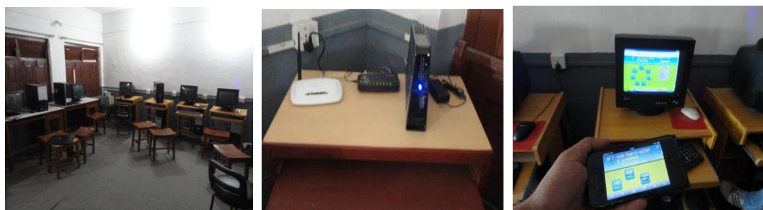
Figure 25: Installation of offline server in one of the public school to allow local access to digital library (E-Pustakalaya) (Source: Author)
