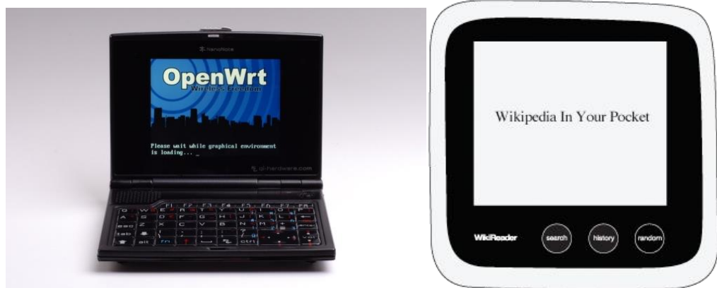
Figure 1a. Ben Nanonote - an ultra-small form factor copyleft computing device which has 336 MHz XBurst CPU, 3.0” display and 2GB NAND flash memory. Figure 1b. Wikireader – offline handheld reading device.
