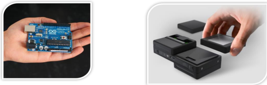
Figure 11: Examples of copyleft hardware (Arduino: electronics prototyping platform and BUG Platform: prototype & produce wireless devices)
