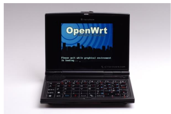
Figure 10: Ben Nanonote - an ultra-small form factor copyleft computing device which has 336 MHz XBurst CPU, 3.0” display and 2GB NAND flash memory
