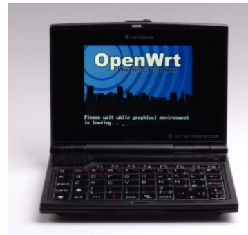
figure 1. Ben Nanonote- 3.0" color TFT display, 336 MHz processor & 2GB of flash memory; an ultra-small form factor Copyleft device by Qi Hardware http://sharism.cc/
