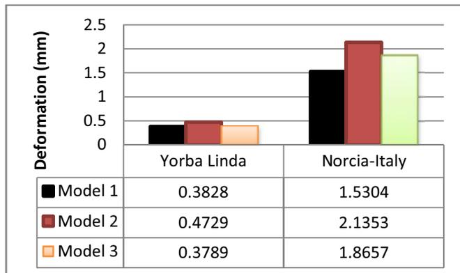
Fig. 11 Maximum directional deformation under 'empty' condition
