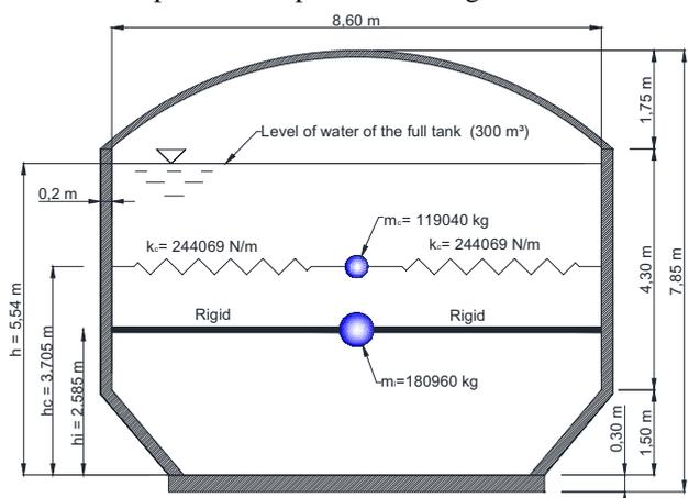
Fig. 5 Modelled water tank
