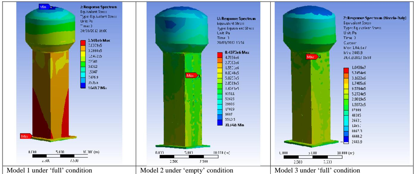
Fig. 13 Von-Mises stress distribution (Pa)
