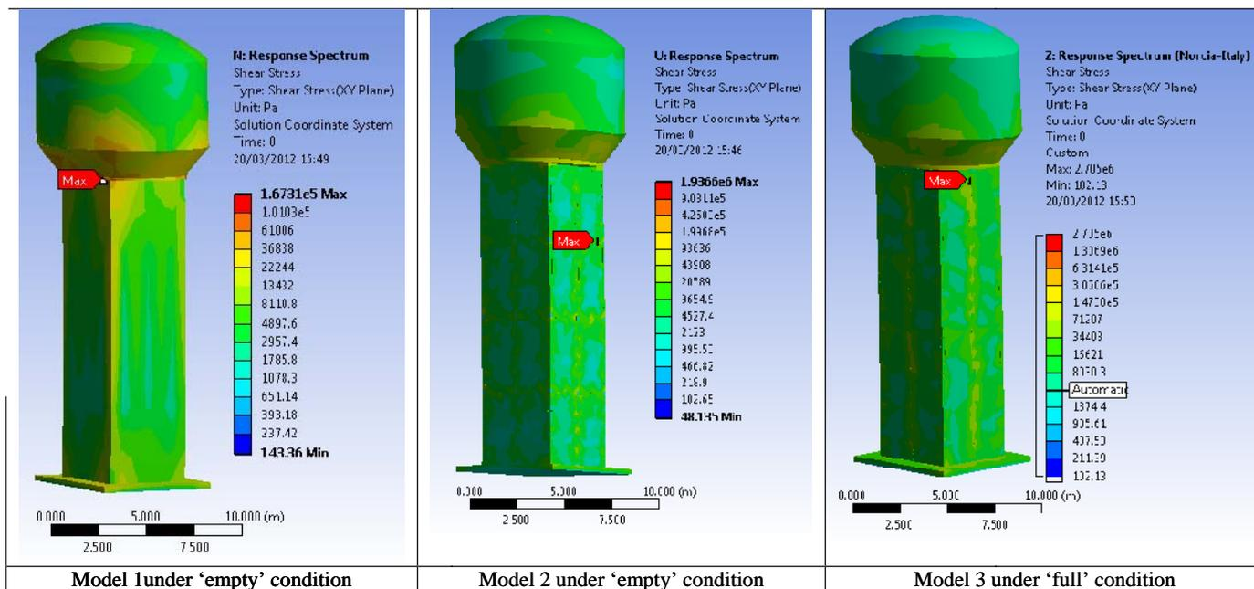
Fig. 12 Shear Stress in XY plane distribution (Pa)
