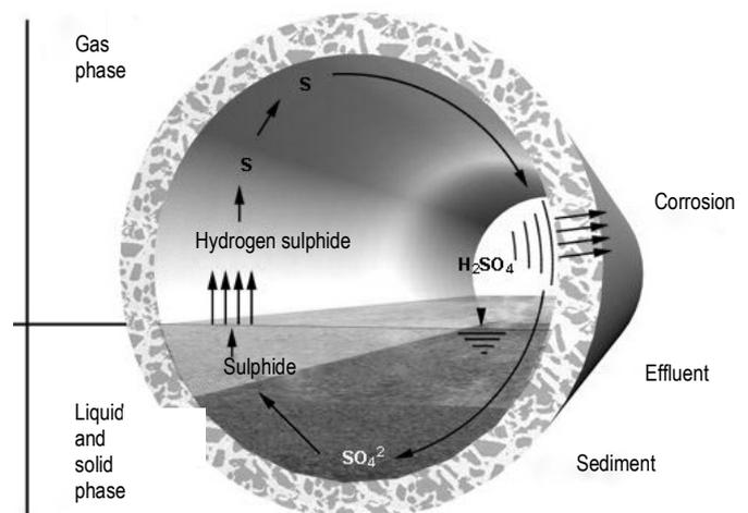
Fig. 1 Microbially induced concrete corrosion in sewer [19]
