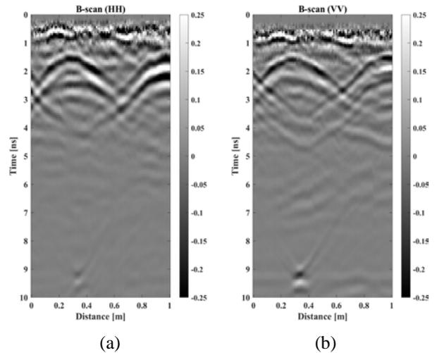
Fig. 2. Post-processed B-scan GPR profile of tree trunk; (a) HH channel B-scan; (b) VV channel B-scan.
