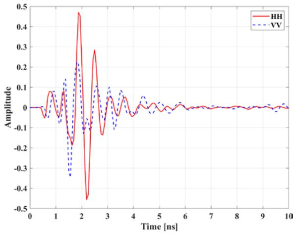
Fig. 3. A-scan of reflection signal obtained at the hyperbolic curve peak.
