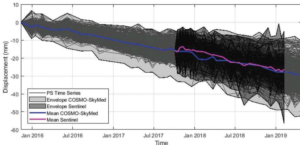
Figure 3. Comparison between displacement time series of PSs within the investigated area (i.e., the yellow rectangular area in Figure 2) for both Sentinel and COSMO-SkyMed data. The envelopes represent areas of maximum and minimum variations of each averaged displacement value across the period analysed.
