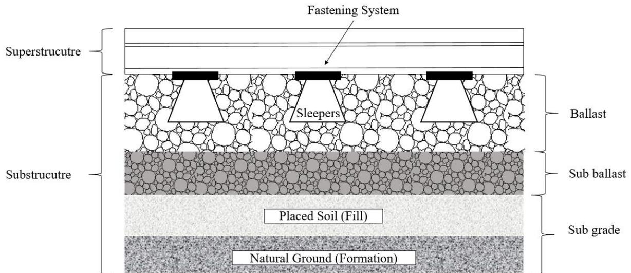
*Figure 1 – Cross-section layout for a ballasted railway*
