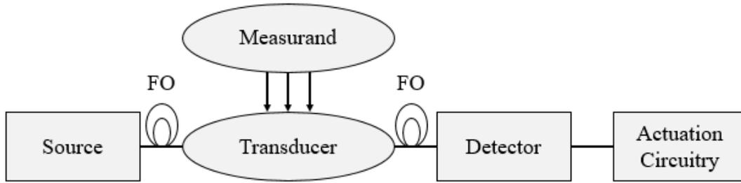
Figure 9 – A schematic system of OFSs
