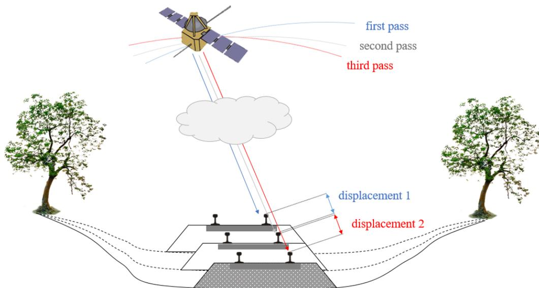
*Figure 13 – Layout of a displacement detection by the InSAR technique. Several images are collected on the same area. Displacements are measured through the variation of the sensor–target distance across the images.*
