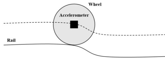
Figure 6 – Layout of inertial track measurements at the longitudinal level
