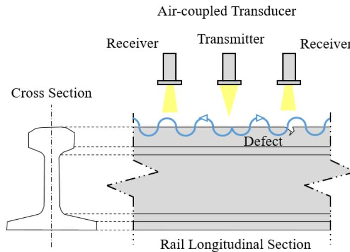
Figure 7 – Illustration of the air-coupled guided wave transducers
