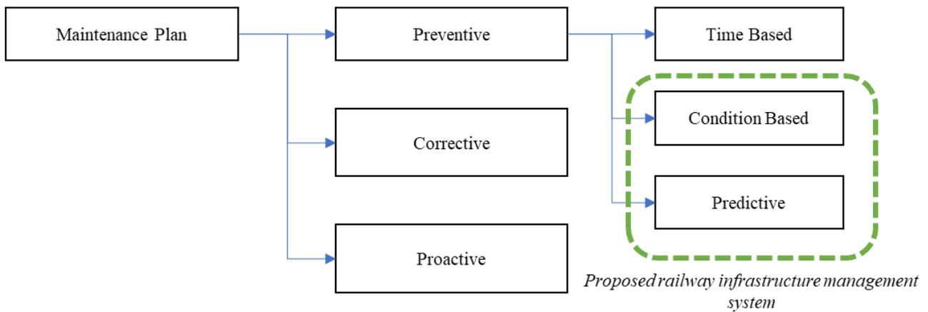
*Figure 15 – Ordinary maintenance plan framework [122]*
