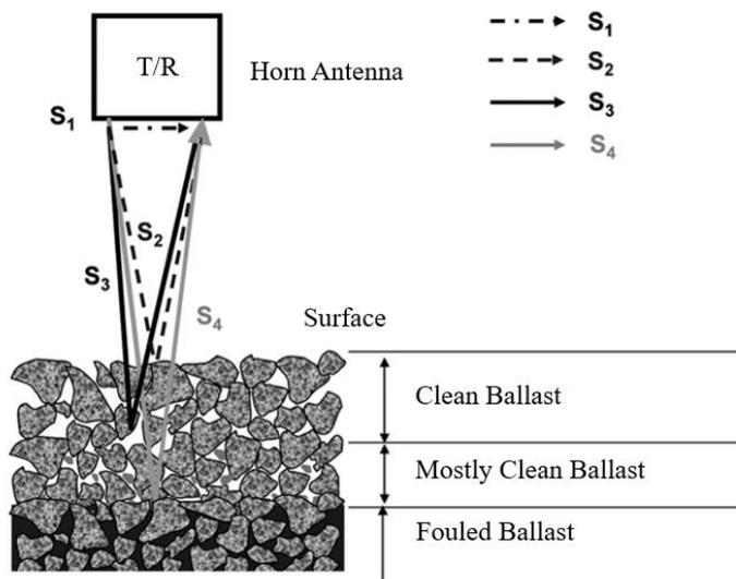
Figure 10 – EM wave propagation in a ballast section
