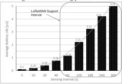
Fig. 3. Average battery life achievable assuming 14 dBm transmission power
