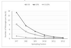
Fig. 4. Maximum number of messages acheivable per day with different LoRa settings considering regional duty cycle restrictions
