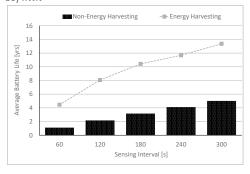
Fig. 9. Average battery lifetime comparison of plain and energy harvesting industrial scenarios employing LoRaWAN
