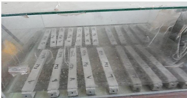
Fig. 10. Setup for sulfate attack test
