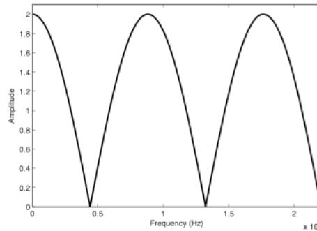
Figure 3 Typical frequency response of a comb filter.
