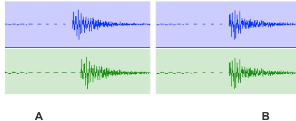
Figure 4 An example of nudging audio regions in an audio editor to compensate for delays that cause comb filtering showing delayed (A) and compensated (B) signals.
