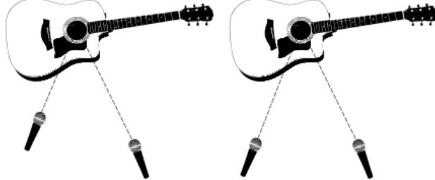
Figure 5 A representation of the effect of using delay compensation to reduce comb filtering.
